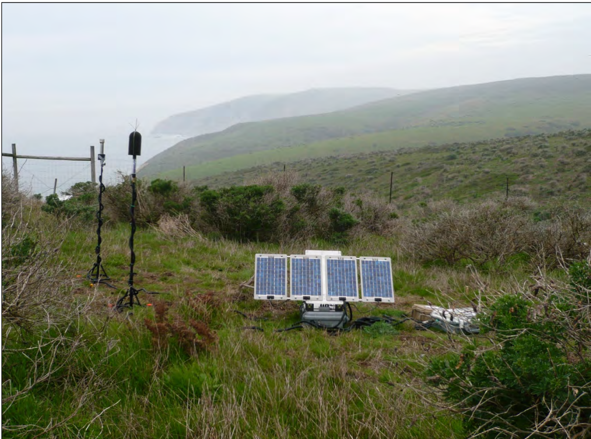
Figure 13. NoiseLogger™ system deployment: Site PORE003.
