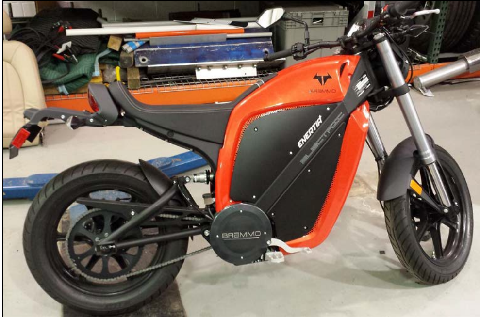
Figure 2. 2012 Brammo Enertia Electric Motorcycle Tested (Source: VRTC)
