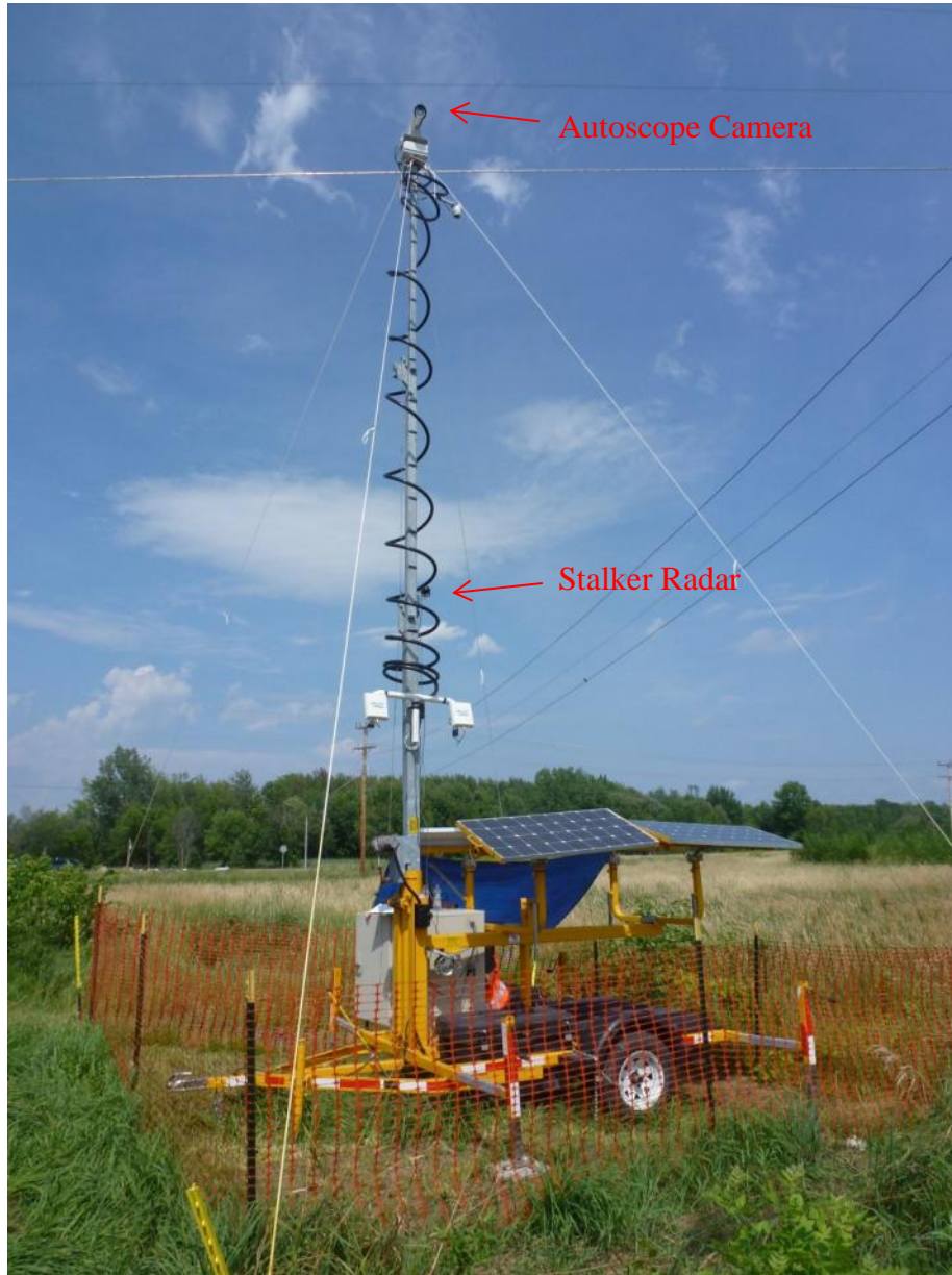
Figure 2. The FRA Mobile Driver Feedback Device Deployed at the Lakewood Drive Grade Crossing in Swanton, Vermont
