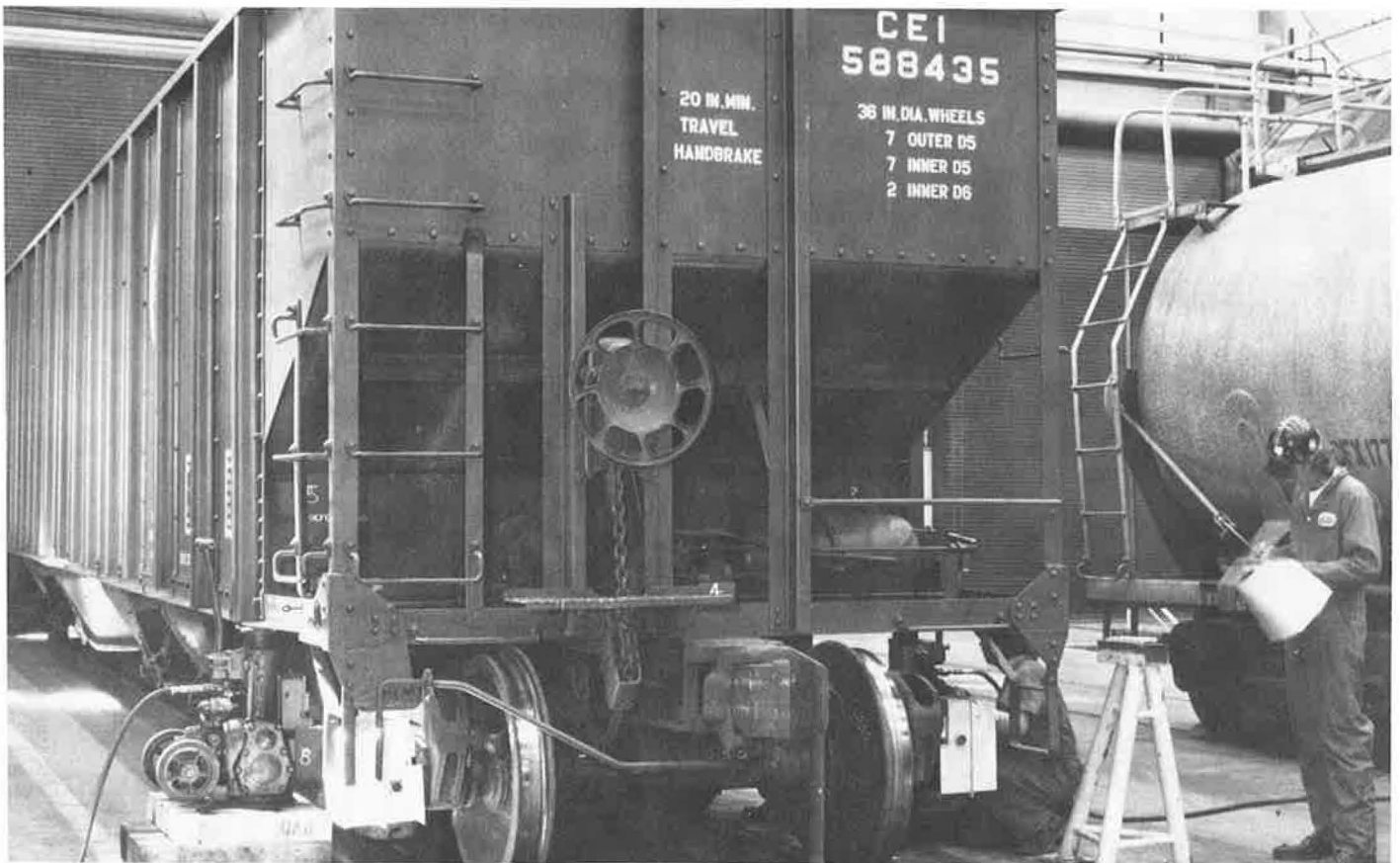
Detailed inspection of all FAST consist cars yields measurement data for studies of car component performance and cost-effectiveness.
