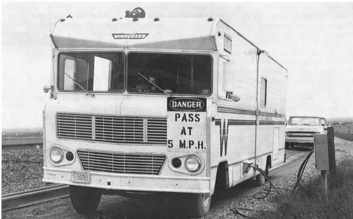
Data van used for recording dynamic measurements from roadbed sensors via wayside junction box.
