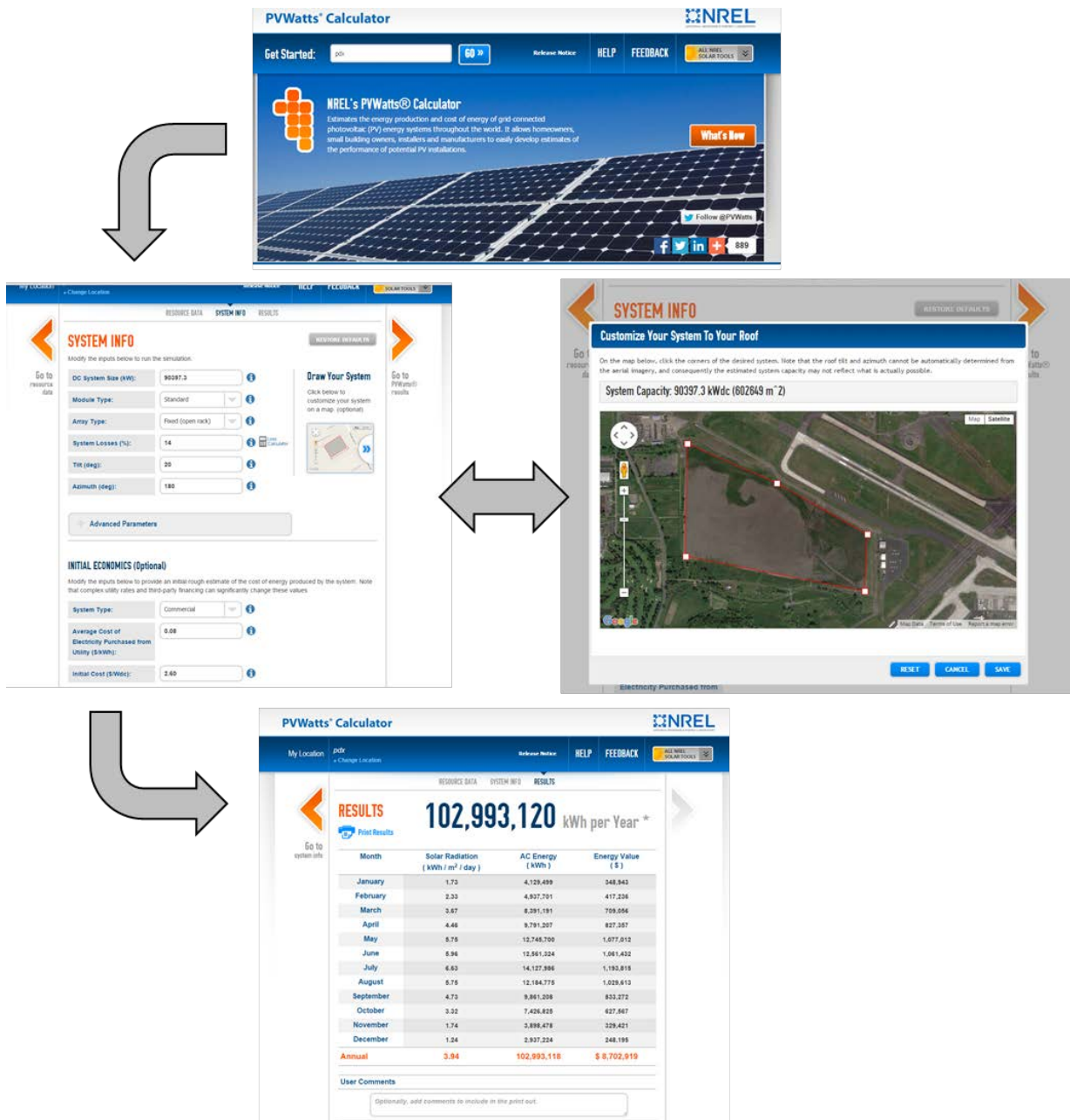
Figure 15. Steps for Estimating Potential Solar PV Output from an Airport Parcel Using PVWatts
