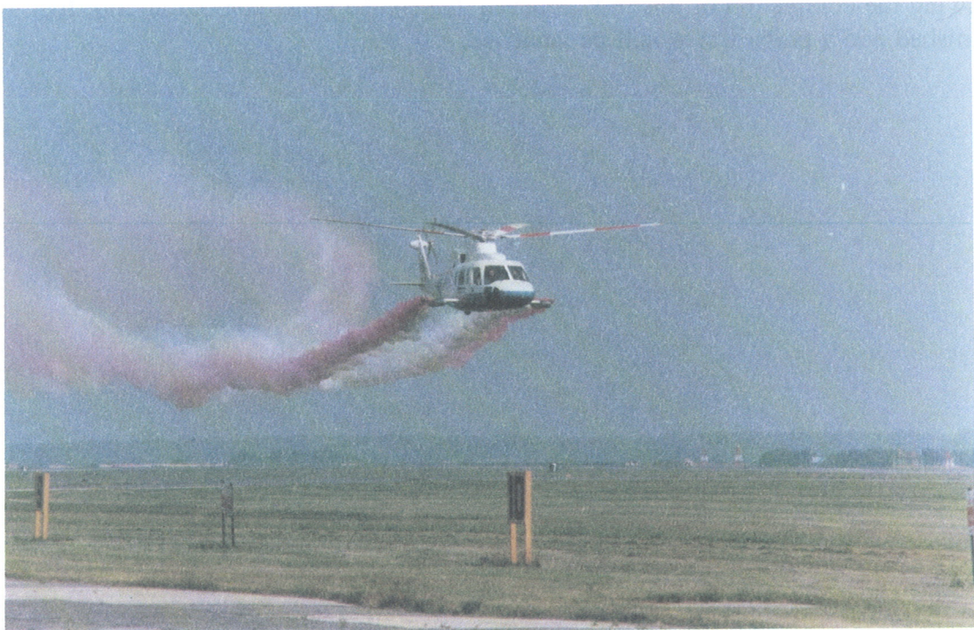
FIGURE 2-9. S-76A WAKE VORTEX FLOW
