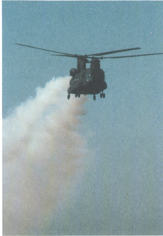
FIGURE 2-4. CH-47D WAKE VORTEX FLOW VISUALIZATION SYSTEM
