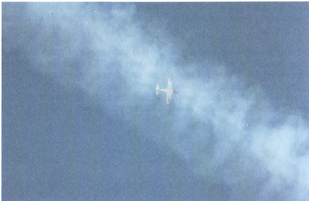
FIGURE 5-3. PROBE TEST (NOTE PROBE AIRCRAFT EXCURSION IN THE VORTEX CORE)
