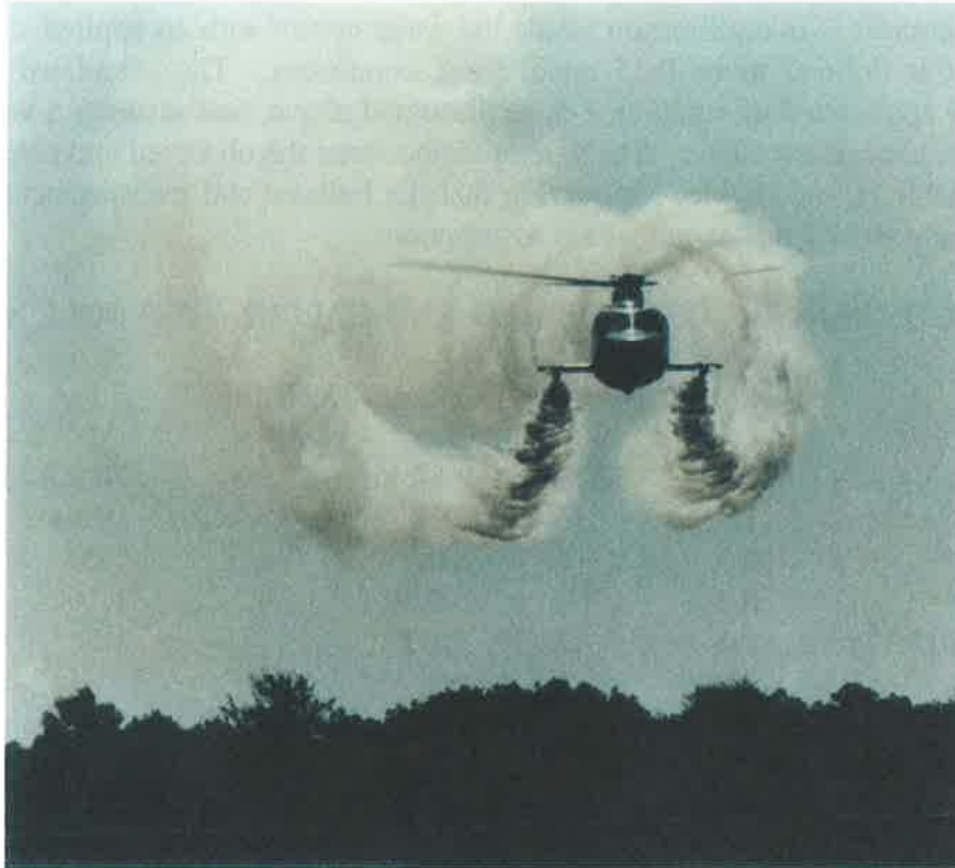
FIGURE 6-7. S-76A WAKE VISUALIZATION
