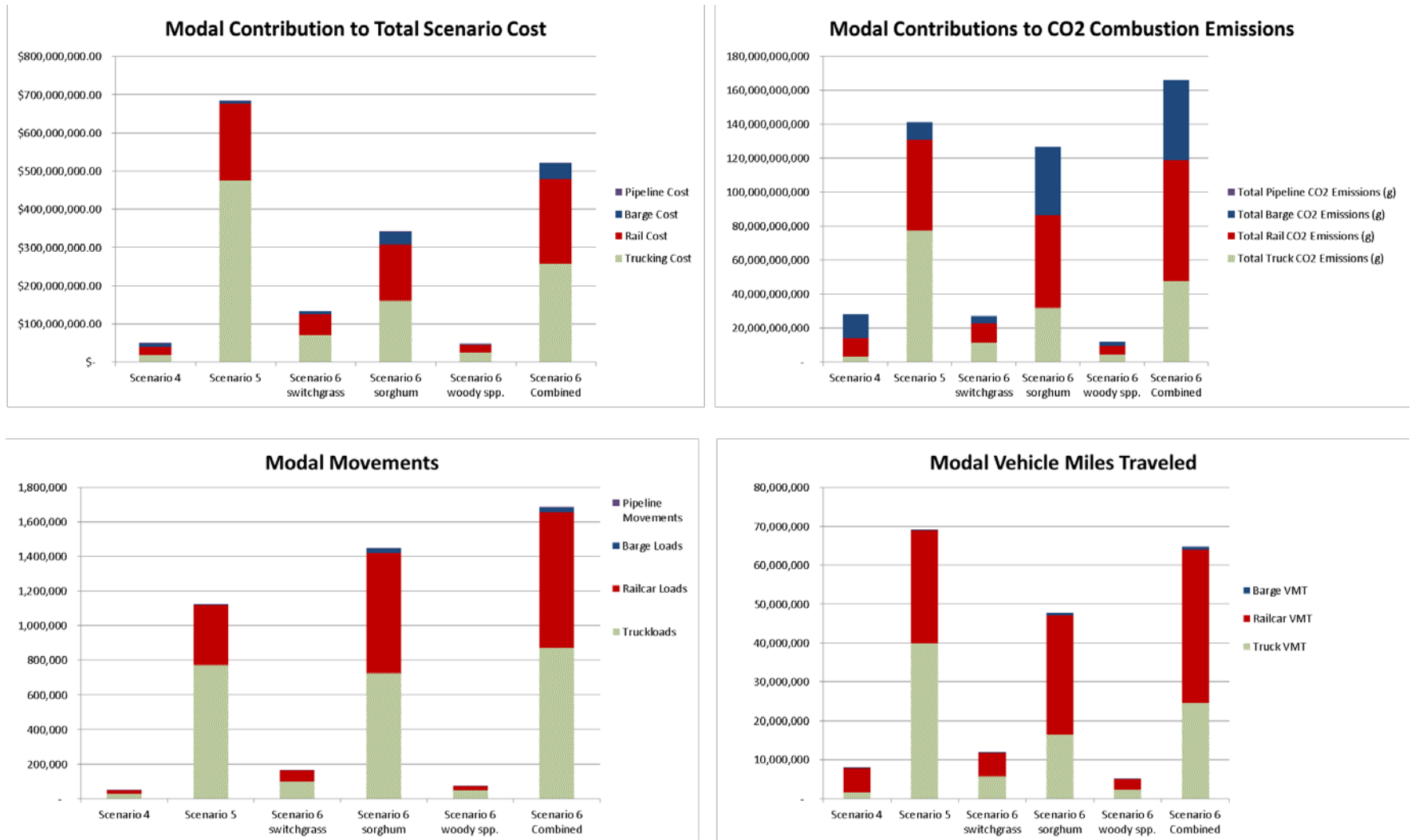
Figure 12: Modal contribution to Scenario Costs, CO 2 Combustion Emissions, Movements (e.g., truckloads, etc.), and vehicle miles traveled (VMT) for Scenarios 4-6. Note that pipeline contribution to total cost is underestimated due to missing base rate values for some routes.
