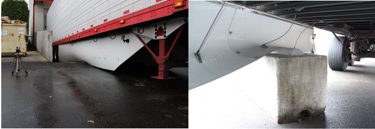
Figure 2-13: Aerodynamic Trailer Skirt Survivability to Impacts 351
