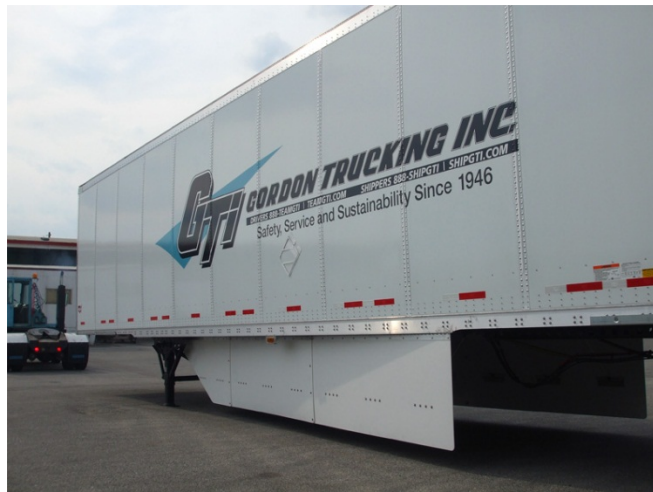
Figure 4-5: Trailer Skirt Made From Resilient Composite Material 451
