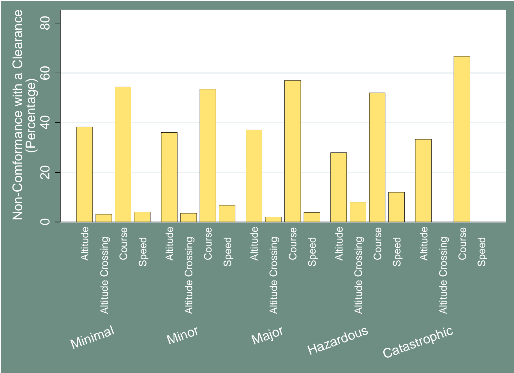
Figure 65 - Distribution (Percentage) Non-Compliance with a Clearance over Severity
