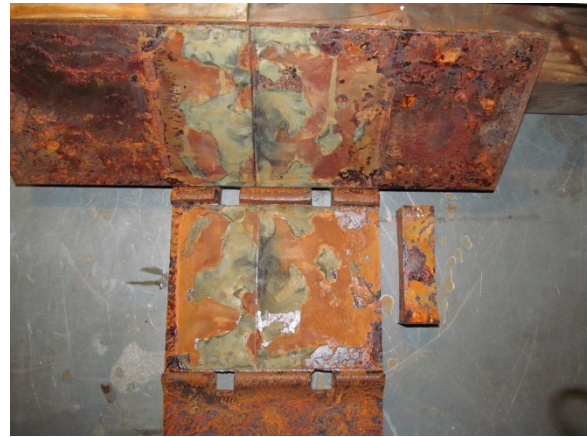
Fig. A-2. Week 1 – PD after Humidity
