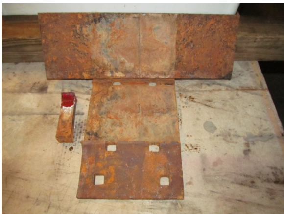
Fig. A-11. Week 3 – ALL after Salt Water
