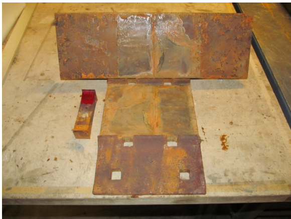
Fig. A-9. Week 2 – ALL after Salt Water
