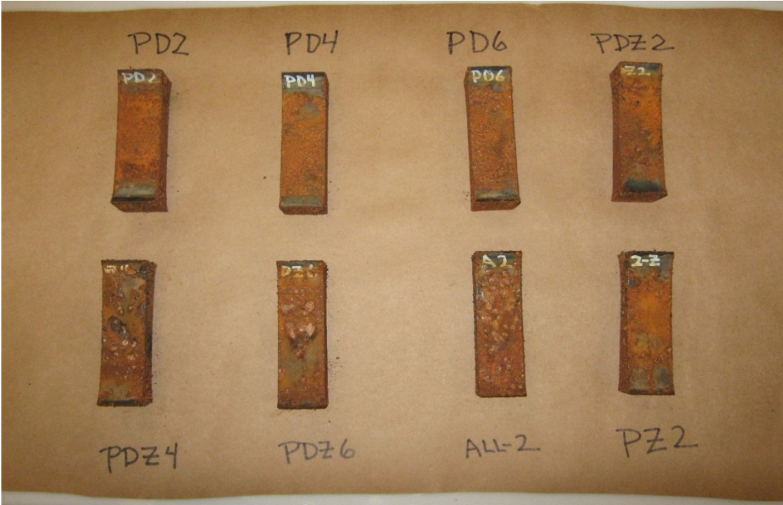
Figure 19. Tops of Samples after 3-Week Corrosion Cycle
