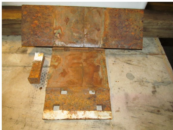
Fig. A-5. Week 3 – PD after Salt Water
