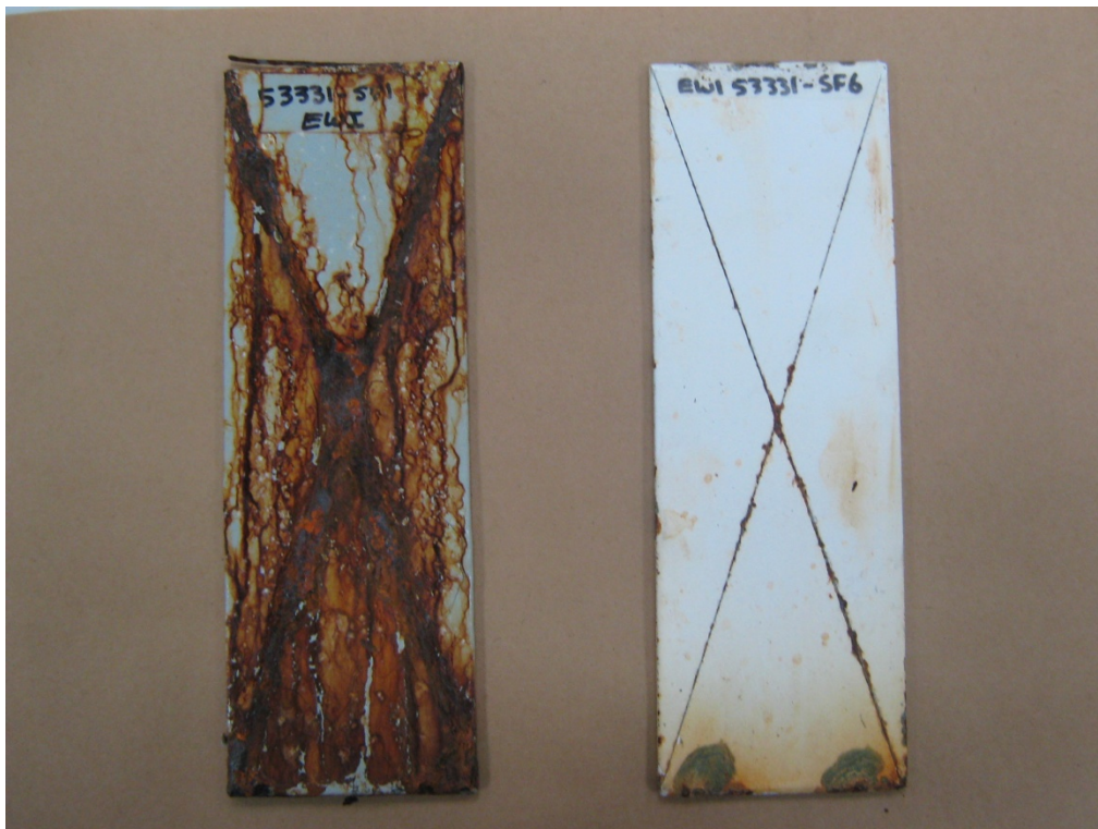
Figure B-2. EWI (left) and EonCoat® (right) after 5000 Hours, Scribed to Metal
