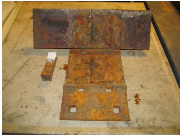
Fig. A-3. Week 2 – PD after Salt Water
