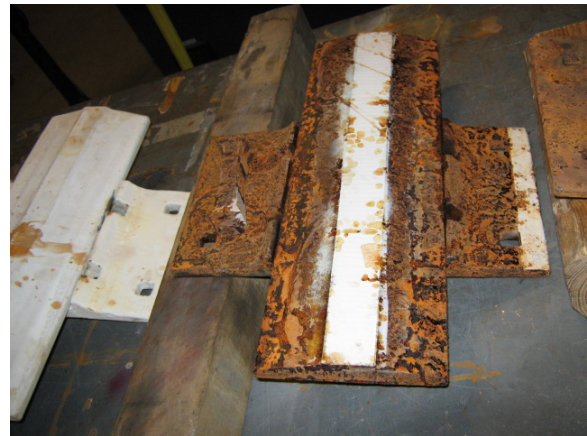
Fig. A-4. Week 2 – PD after Humidity
