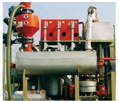
Biofuels can be produced from oilseeds such as sunflower, flax, and safflower (top). A mobile, pilot-scale microwave-assisted pyrolysis system like the one shown here lets the University of Minnesota perform biofuels research outside of the laboratory (bottom).
