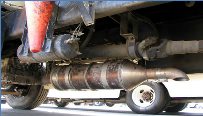
Figure 14: Image of a refuse truck is outfitted with a diesel particulate filter. (Courtesy of FHWA)
