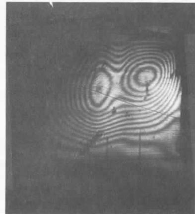
Figure 8. Holographic Interferogram of a Rubber/Cord Specimen with a Ply Overlap
