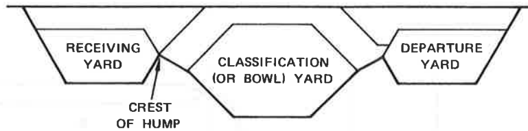
FIGURE 51 TANDEM OR IN-LINE ARRANGEMENT OF SUBYARDS
