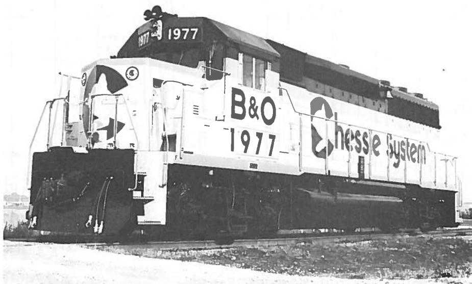
FIGURE 7 GENERAL PURPOSE, 3000 HORSEPOWER, FOUR-AXLE DIESEL-ELECTRIC LOCOMOTIVE
