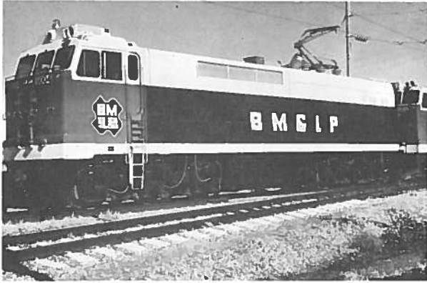
FIGURE 19 BLACK MESA AND LAKE POWELL E60, THYRISTOR ELECTRIC LOCOMOTIVE, 6000 HP, 50 KV, 60 HZ
