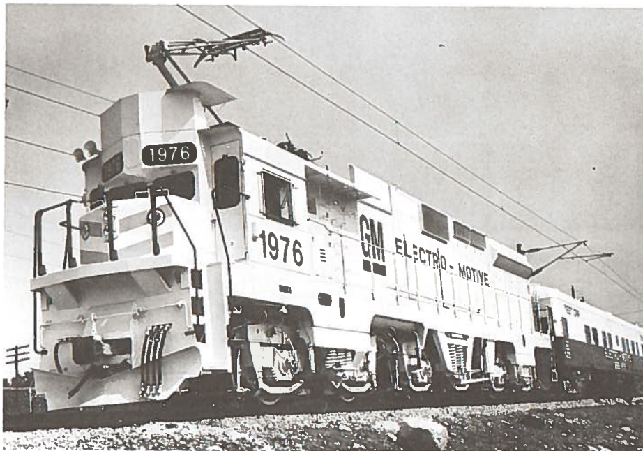
FIGURE 19 GM-10-B 10000 HORSEPOWER ELECTRIC LOCOMOTIVE
