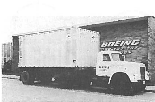
Figure 21 INTERMODAL CONTAINER ON ISO CHASSIS
