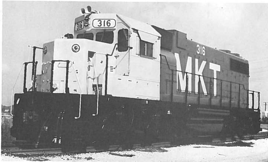
FIGURE 6 GENERAL PURPOSE, 2000 HORSEPOWER, FOUR-AXLE DIESEL-ELECTRIC LOCOMOTIVE
