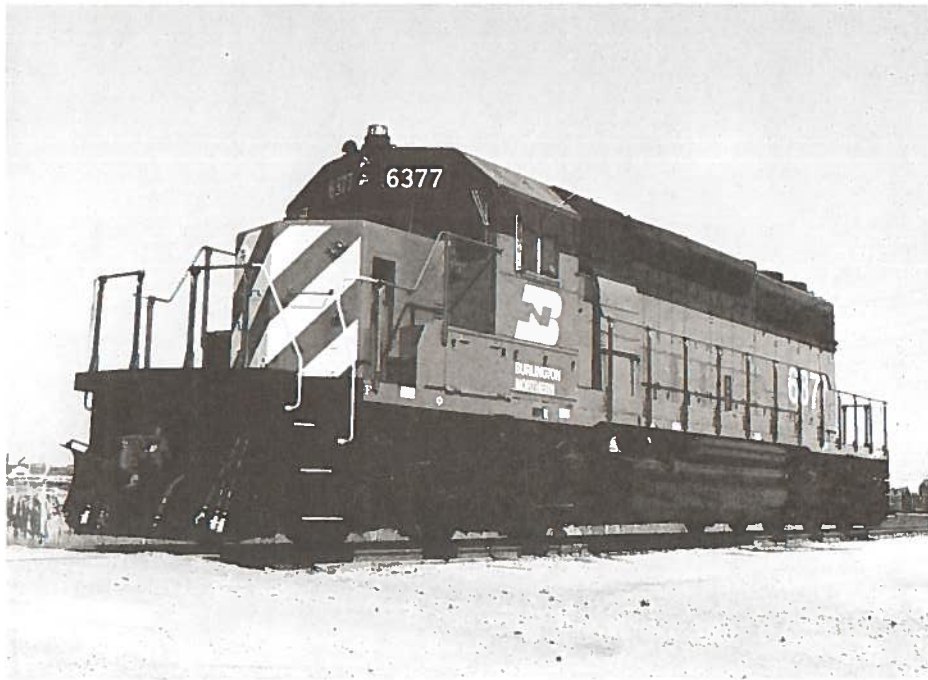
FIGURE 8 HEAVY-DUTY FREIGHT, 3000 HORSEPOWER, SIX-AXLE LOCOMOTIVE
