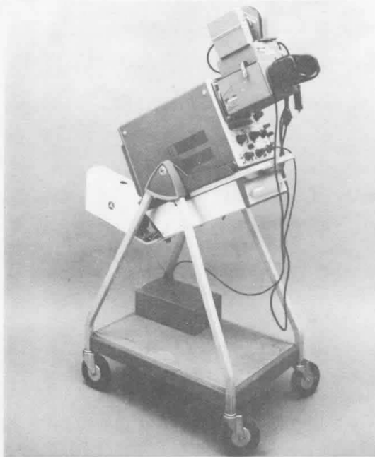
Figure 2. Field Infrared Tire Inspection System (FITIS) Mounted on Scope Cart
