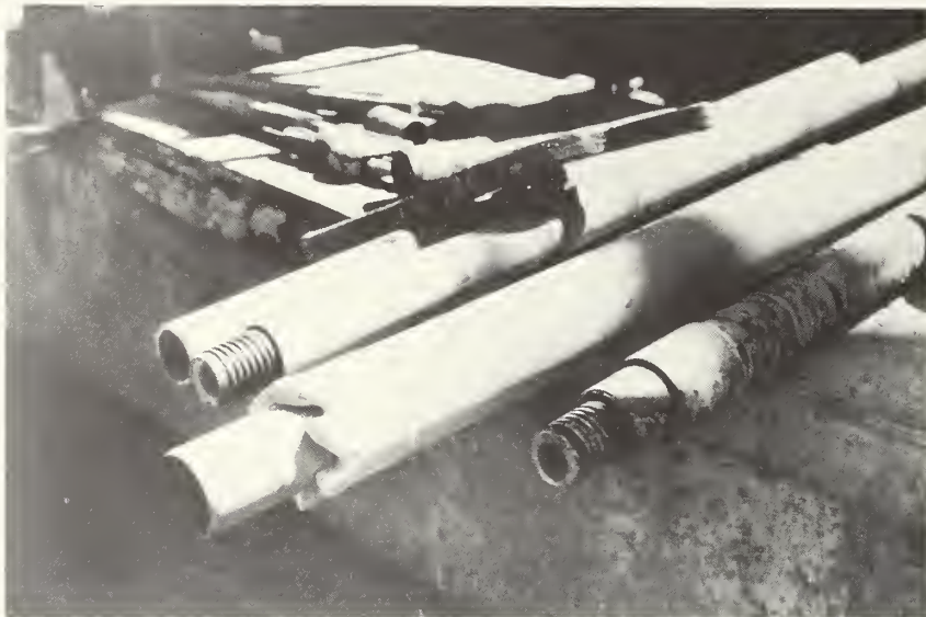
FIGURE 7-24. PITCHER TM SAMPLER WITH PROTRUDING SPRING-LOADED INNER SAMPLE TUBE
