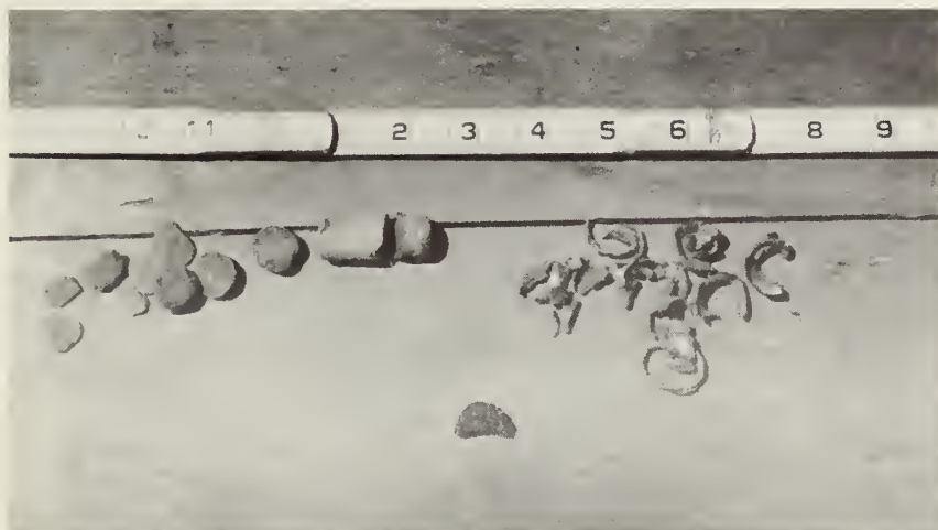
FIGURE 7-43. RWT CORE AND DESTROYED BIT
