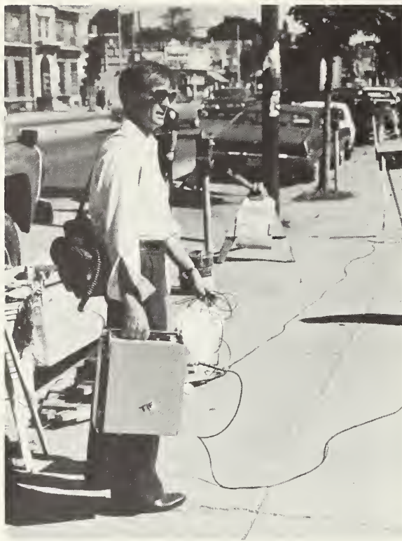
FIGURE 7-63. LIGHTWEIGHT AND PORTABLE SIGNAL ENHANCEMENT SEISMIC EQUIPMENT
