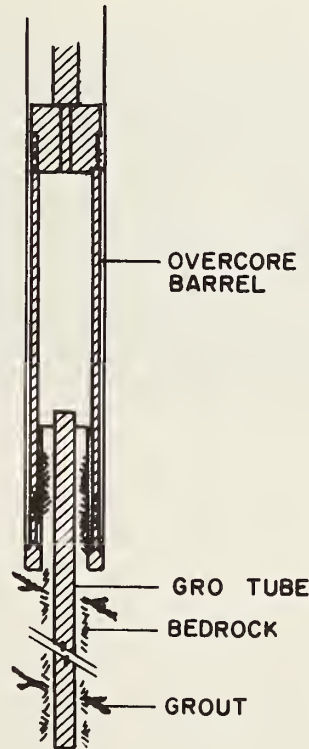
FIGURE 7-37. ISM PHASE III, OVERCORING GROUT REINFORCED GRO TUBE
