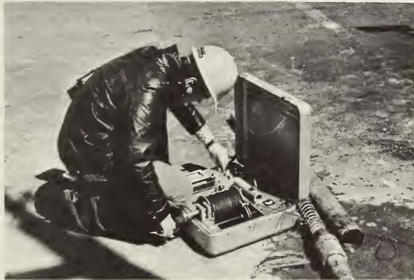
FIGURE 7-57. ELECTRICAL BOREHOLE LOGGING
