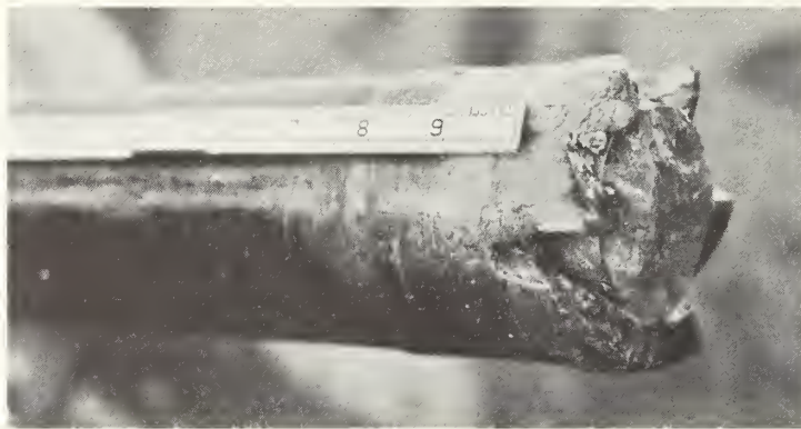
FIGURE 7-26. PITCHER TM SAMPLER WITH CORED BOULDER JAMMED IN SAMPLE TUBE
