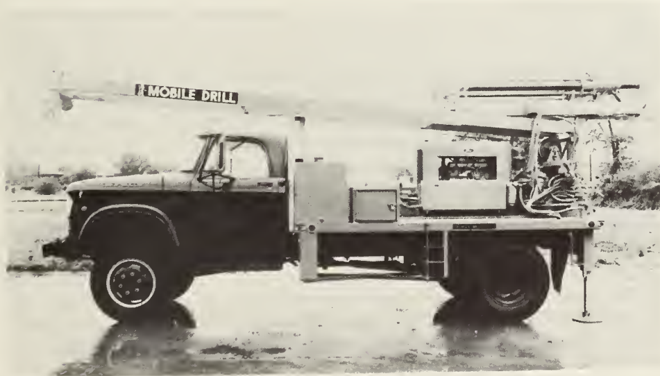
FIGURE 7-5. MOBILE B56 TM DRILL RIG
