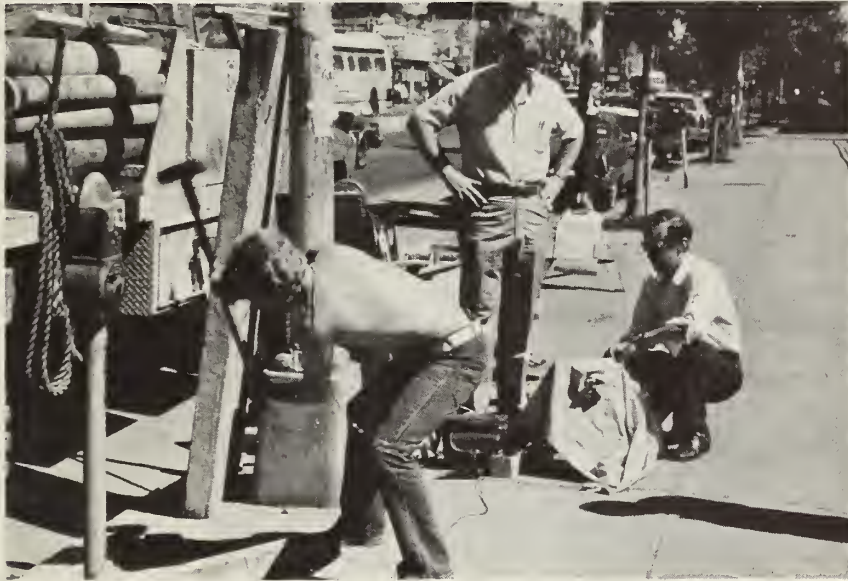
FIGURE 7-62. UTILIZING SIGNAL ENHANCEMENT TECHNIQUES FOR SURFACE SEISMIC REFRACTION SURVEY
