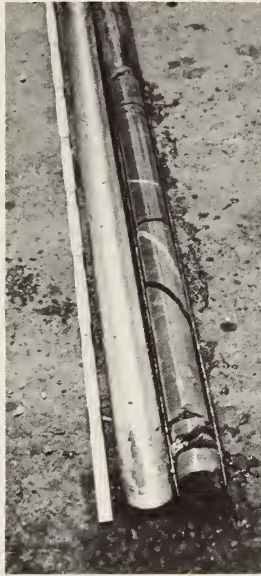
FIGURE 7-32. FULL RECOVERY OF ARGILLITE IN NWD3 TM SPLIT LINER
