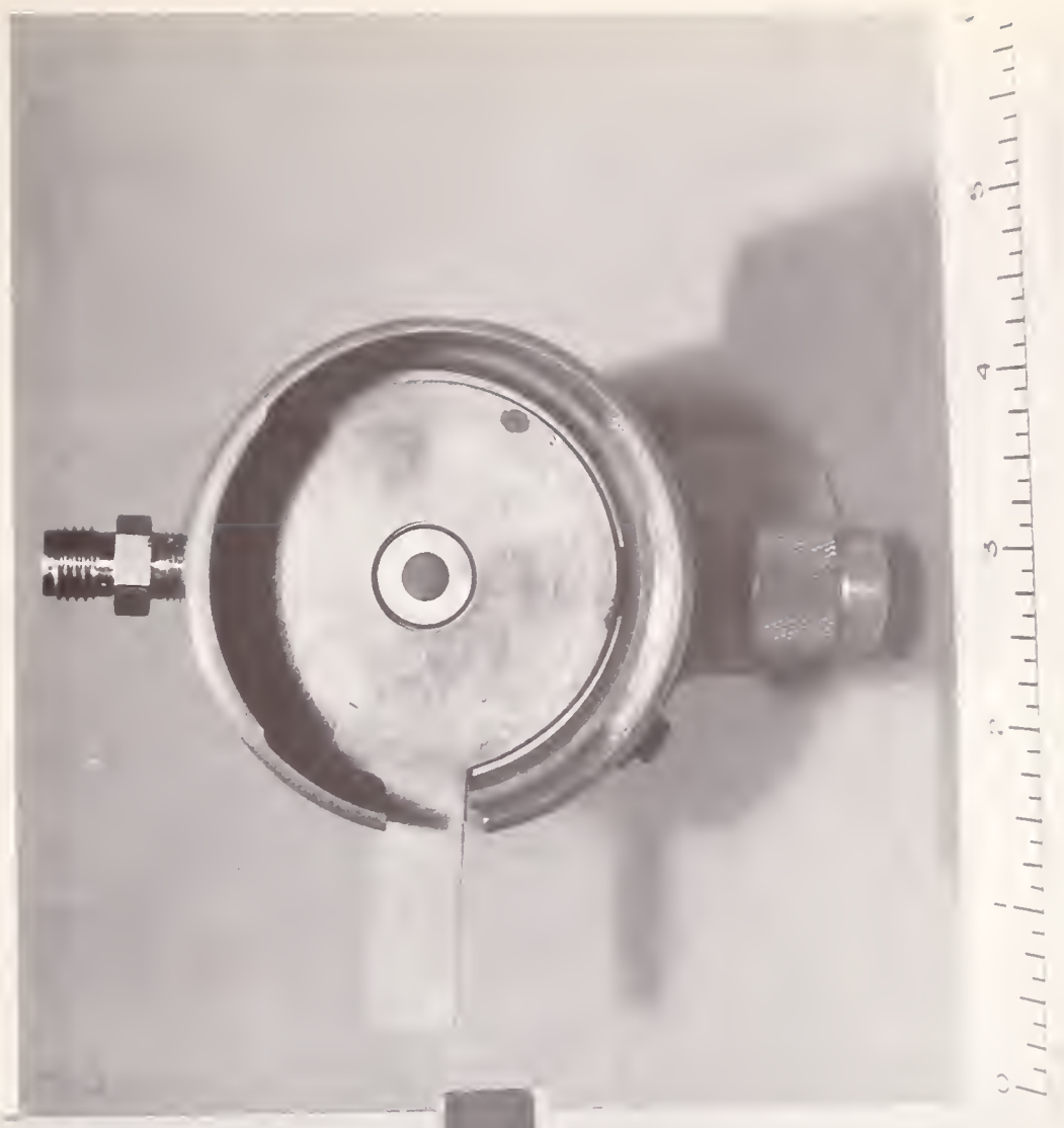
Figure 3. Flowmeter Dual Orifice - Small Orifice, High-Pressure Position
