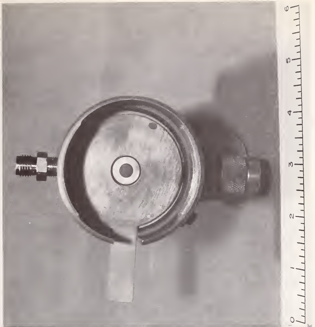
Figure 3-3. Flowmeter Dual Orifice--Small-Orifice, High-Pressure Position
