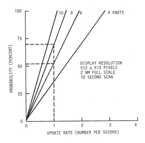
FIGURE A-6. PROBABILITY OF A PILOT DETECTING VESSEL MOVEMENT
