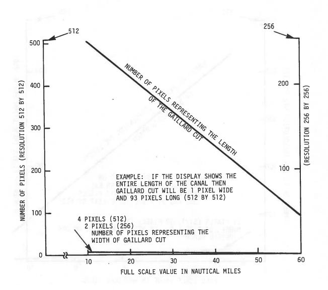
FIGURE A-1. DISPLAY SCALE 60 TO 10 NAUTICAL MILES
