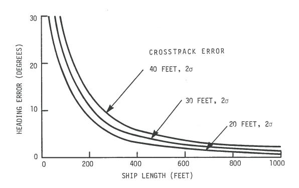
FIGURE A-3. HEADING ERROR AS A FUNCTION OF SHIP LENGTH
