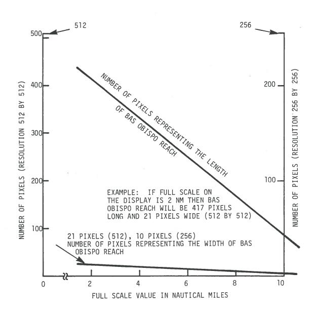
FIGURE A-2. DISPLAY SCALE 10 TO 2 NAUTICAL MILES
