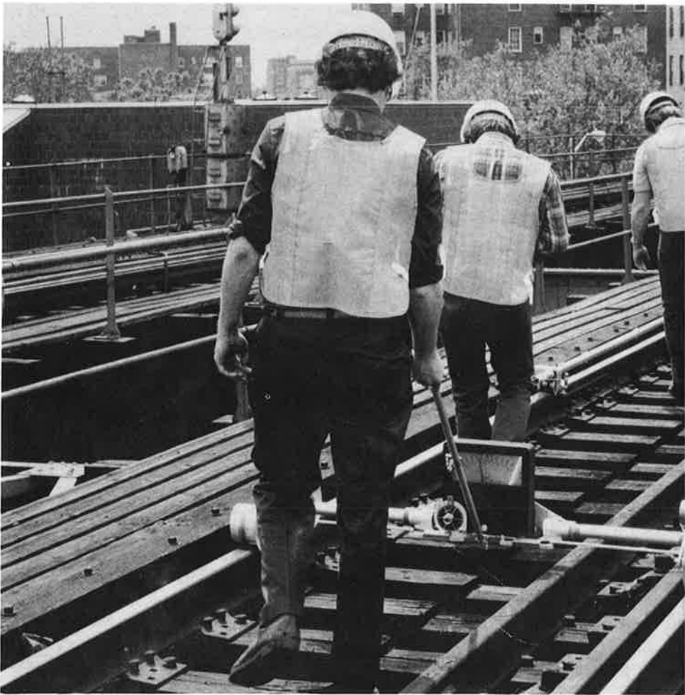
Hand-measurement of track geometry parameters is still widely employed.
