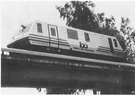
BART's track geometry car is a step towards prioritizing track maintenance automation.
