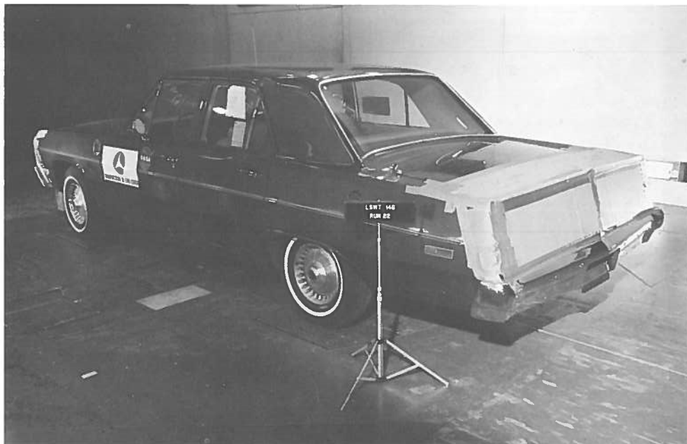
Figure 4. Impala Sedan with Short Nose, Window Fairings and Underpan as Modifications
