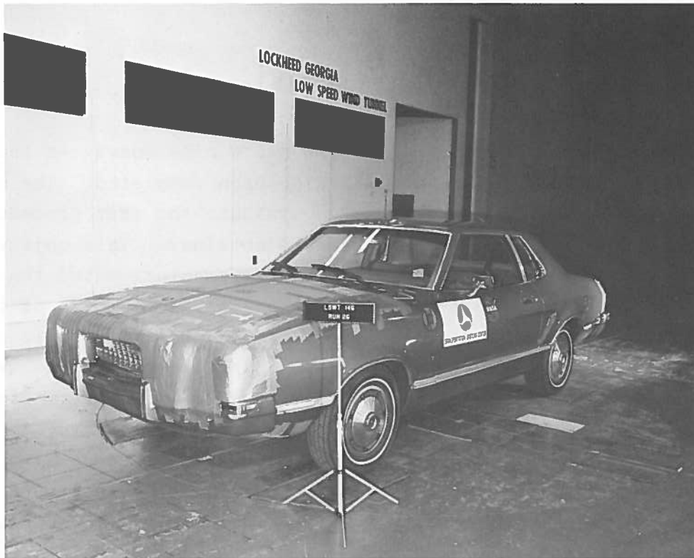
Figure 6. Mustang II with Short Nose, Short Underpan and Square Back as Modifications
