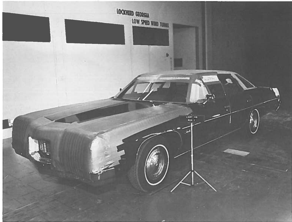
Figure 4. Impala Sedan with Short Nose, Window Fairings and Underpan as Modifications
