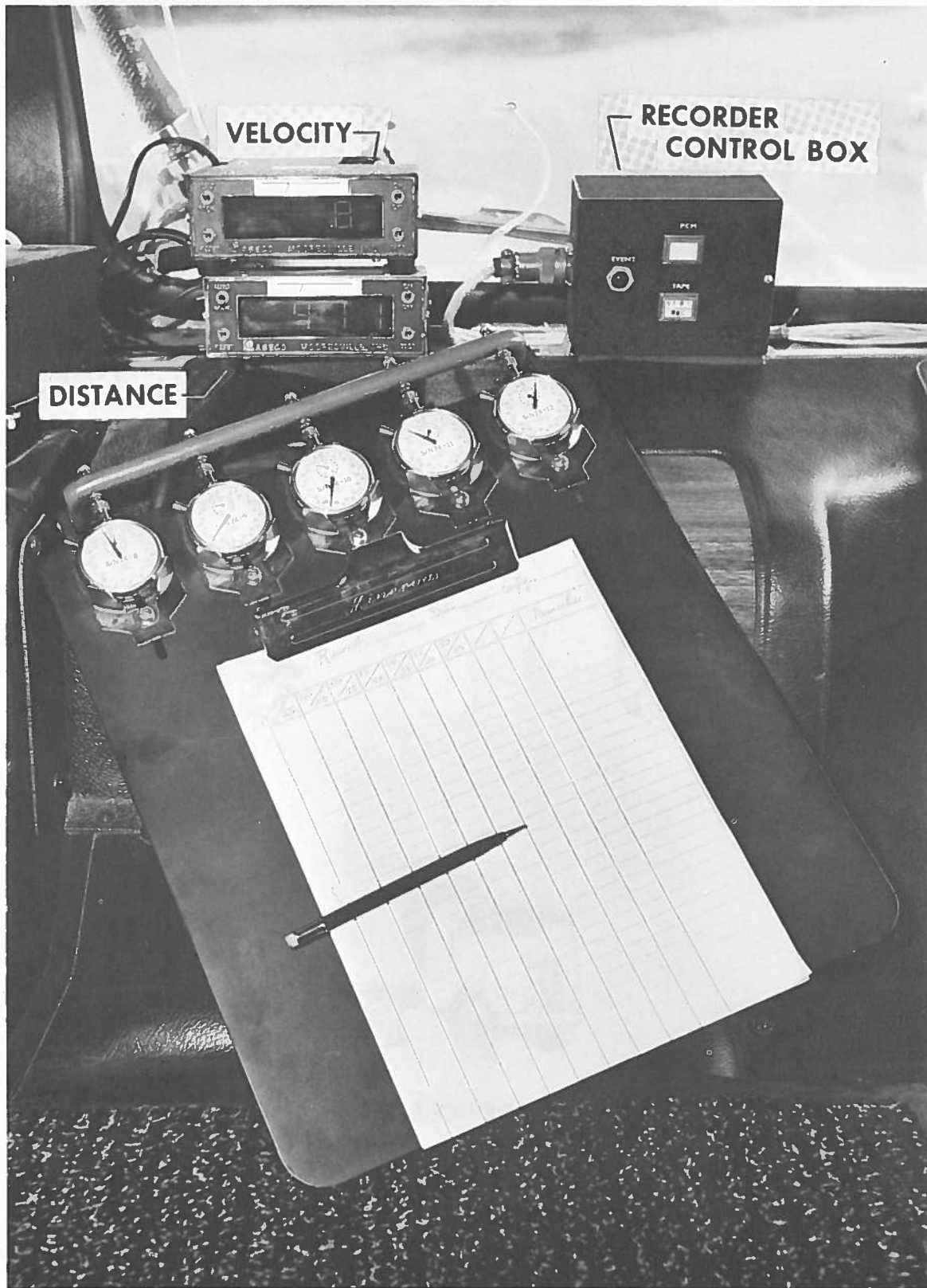
Figure 3. Instrumentation layout inside cab.
