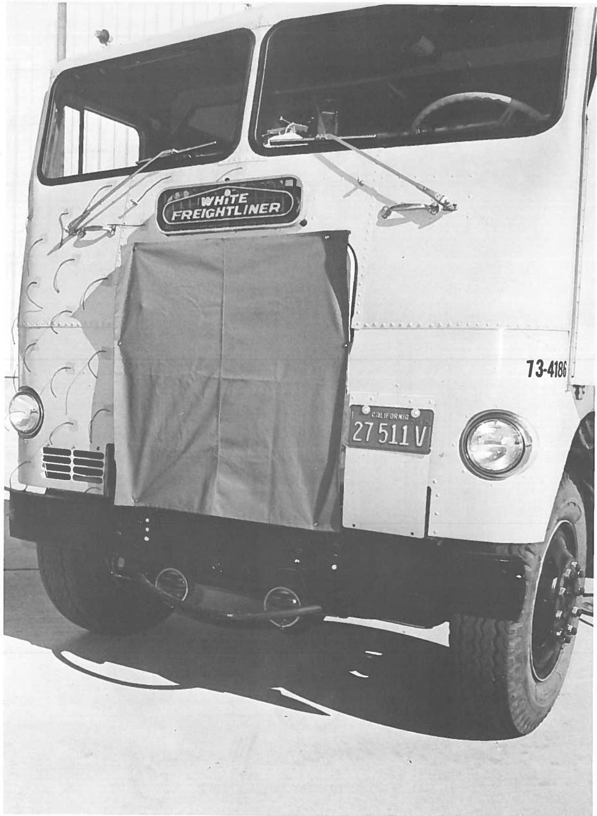
Figure 2. Cover over radiator opening.
