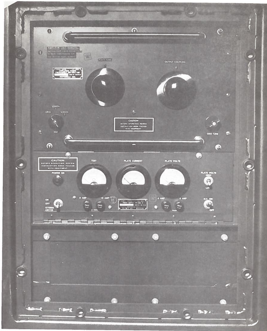
Figure 2-6. Photograph of UHF Power Amplifier
