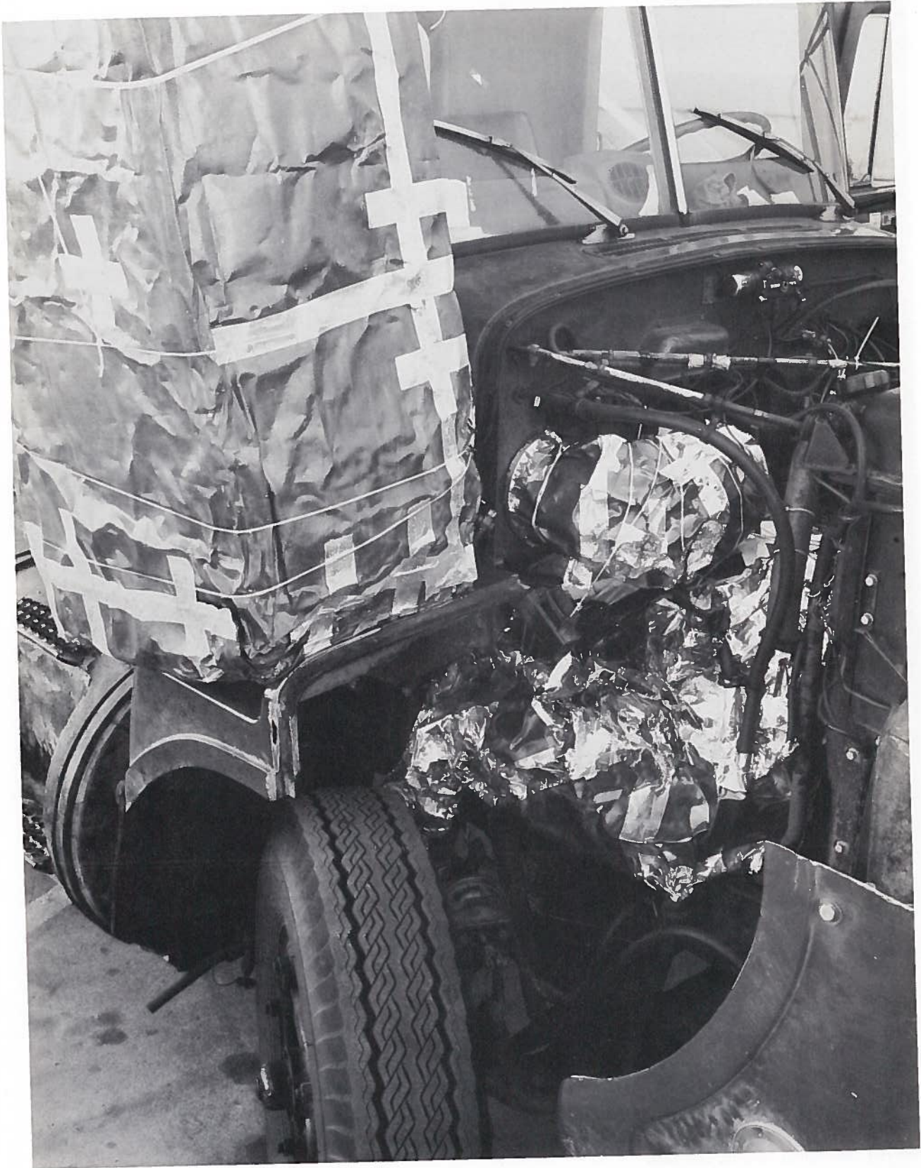
Figure 13. Shrouding Details, Right Side
