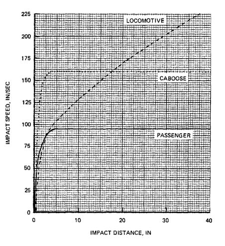
Figure 3–12. Body Impact Velocity vs Distance Traveled
