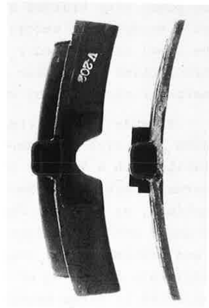
B. Side view—new shoe and simulated wornout shoe.
