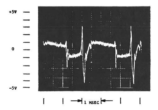
FIGURE 3. RAIL-TO-RAIL INDUCTIVE INTERFERENCE VOLTAGE VS. TIME FOR A MARTA CAR.
