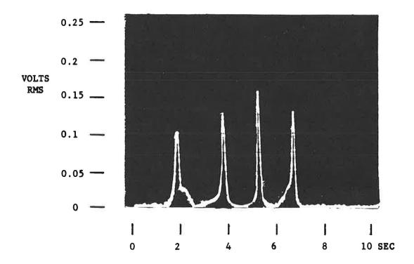
FIGURE 8. AMPLITUDE OF THE INDUCTIVE INTERFERENCE HARMONIC AT 2616 HZ VS. TIME FOR A BART TRAIN.
