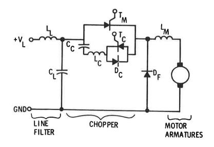
FIGURE 2. A CHOPPER CIRCUIT SHOWING WIRING FOR PROPULSION MODE.
