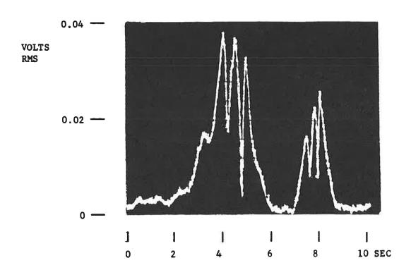
FIGURE 11. AMPLITUDE OF THE INDUCTIVE INTERFERENCE HARMONIC AT 3000 HZ VS. TIME FOR A NYCTA TRAIN.
