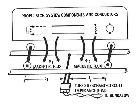
FIGURE 1. CONFIGURATION OF CAR AND SIGNALING EQUIPMENT LEADING TO INDUCTIVE CHOPPER INTERFERENCE.
