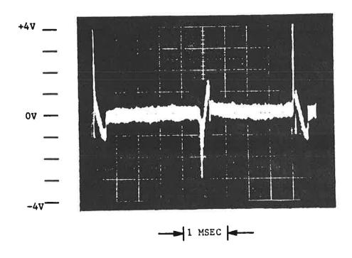
FIGURE 6. RAIL-TO-RAIL INDUCTIVE INTERFERENCE VOLTAGE VS. TIME FOR A BART CAR.
