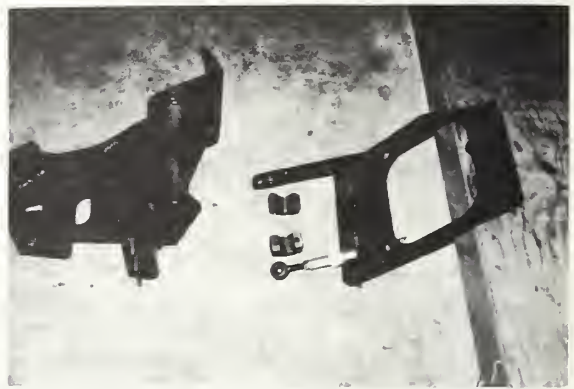
FIG. 4. MIAMI MOD. #1 & (FINAL) RTS MOUNTING BASE COMPONENTS
