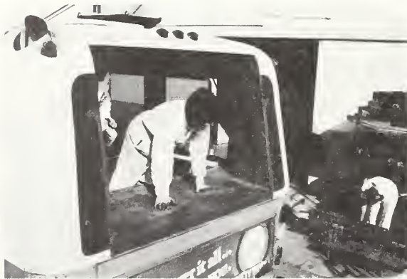
FIG. 17. L.A. MOD. (FINAL) FINISHED OPENING FOR A/C ASSEMBLY
