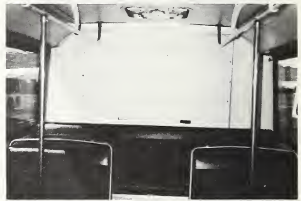
FIG. 13. L.A. MOD. #1 WHITE PLASTIC LAMINATE INTERIOR REAR PARTITION
