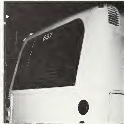
FIG. 8. MIAMI MOD. (FINAL) FIBERGLASS LOUVER PANEL
