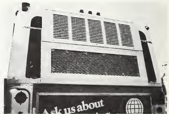
FIG. 20. L.A. MOD. (FINAL) LOUVERED INTAKE GRILL IN FRONT OF CONDENSER FANS (PRIME PAINTED)
