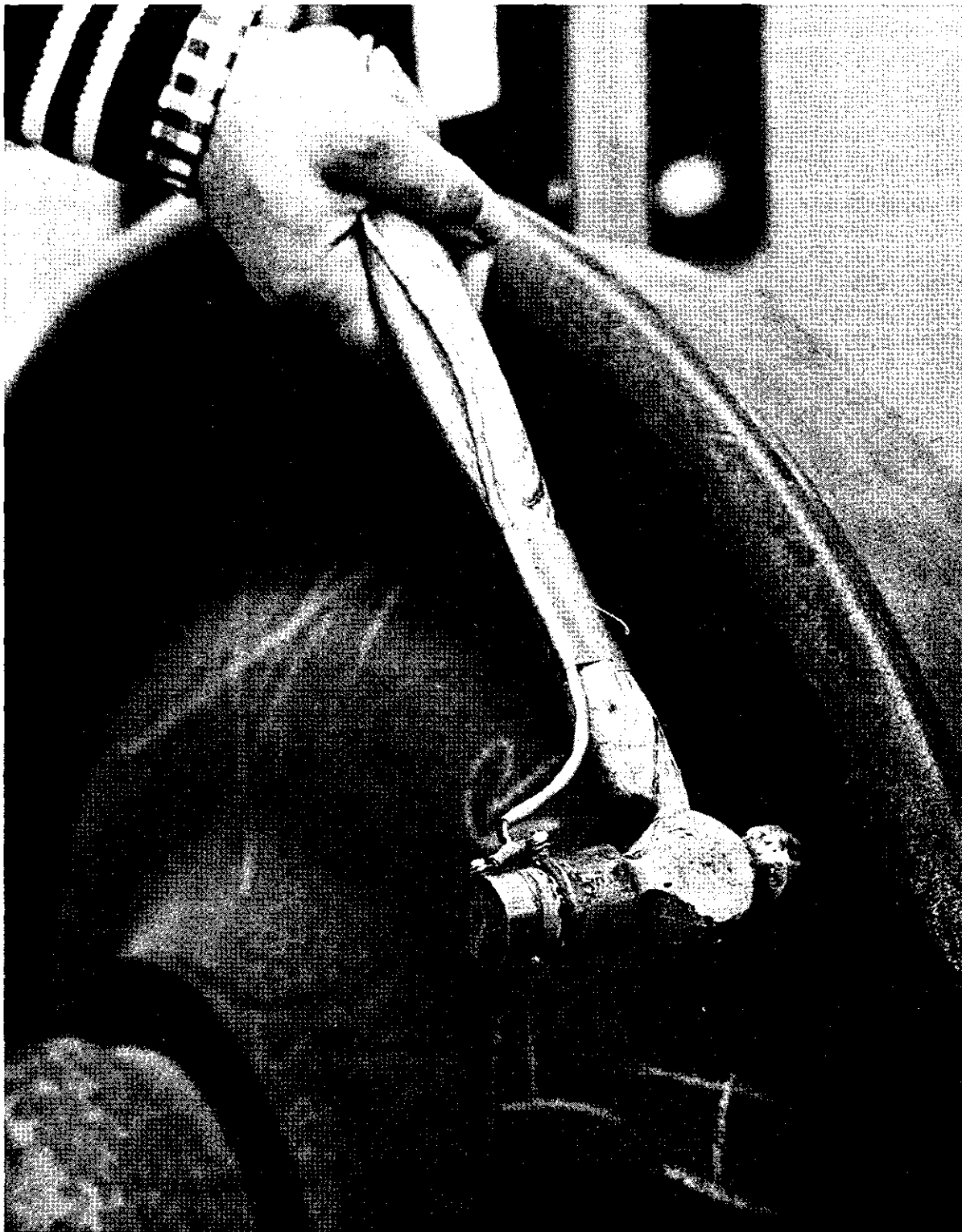
FIG. 4.2.2 VIEW OF THE HAMMER WITH A PZT DISK BETWEEN HAMMER AND CYLINDER TO PROVIDE THE TRIGGERING PULSE ON IMPACT WITH THE TEST OBJECT
