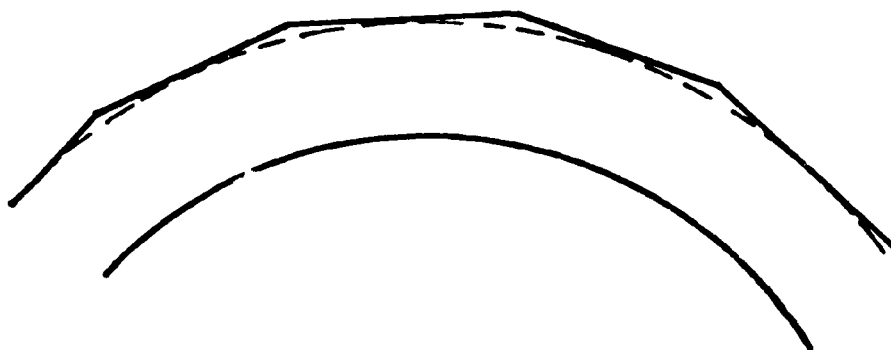
Figure G-5 High Rail Misalignment
