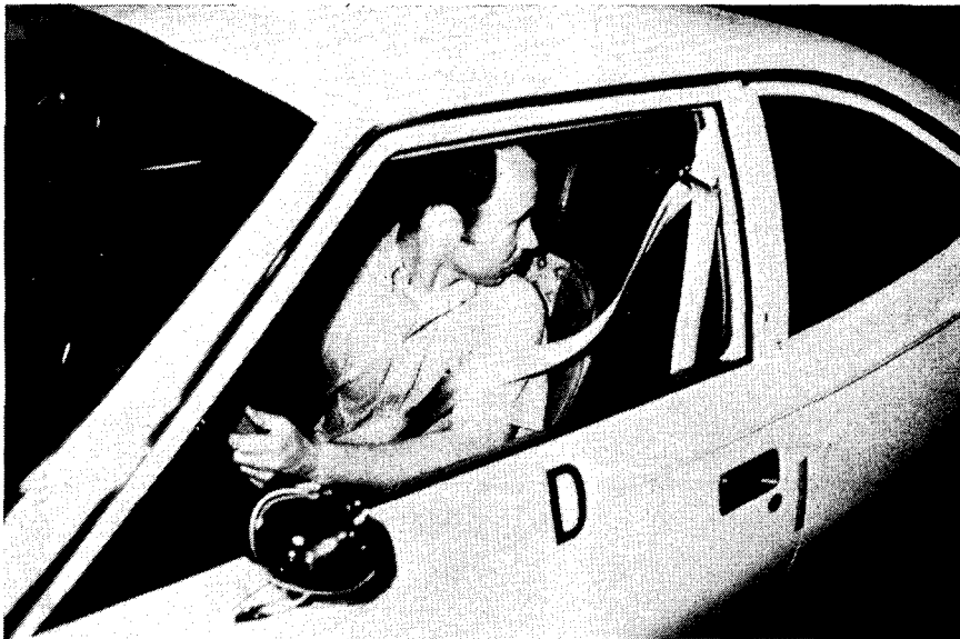
FIGURE 18 Belt Off Shoulder Looking to Rear - Passive Hornet
