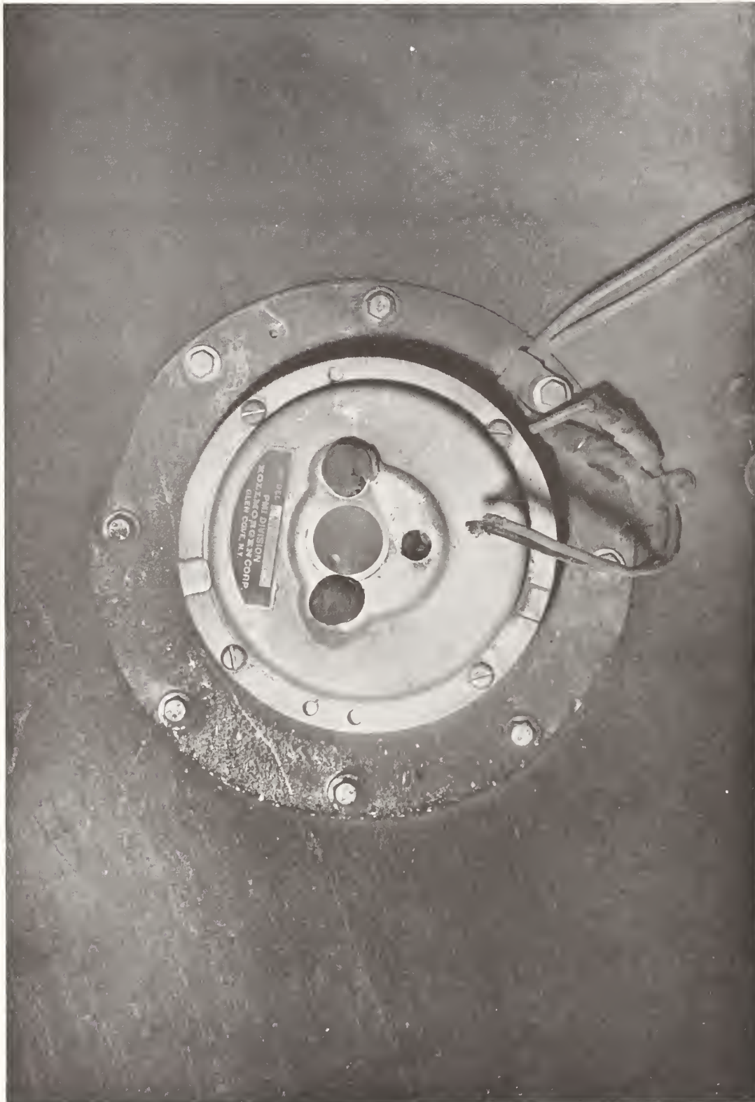
Figure 18. Damage to ASL Electric Ramp Motor Incurred During Ride Tests.
