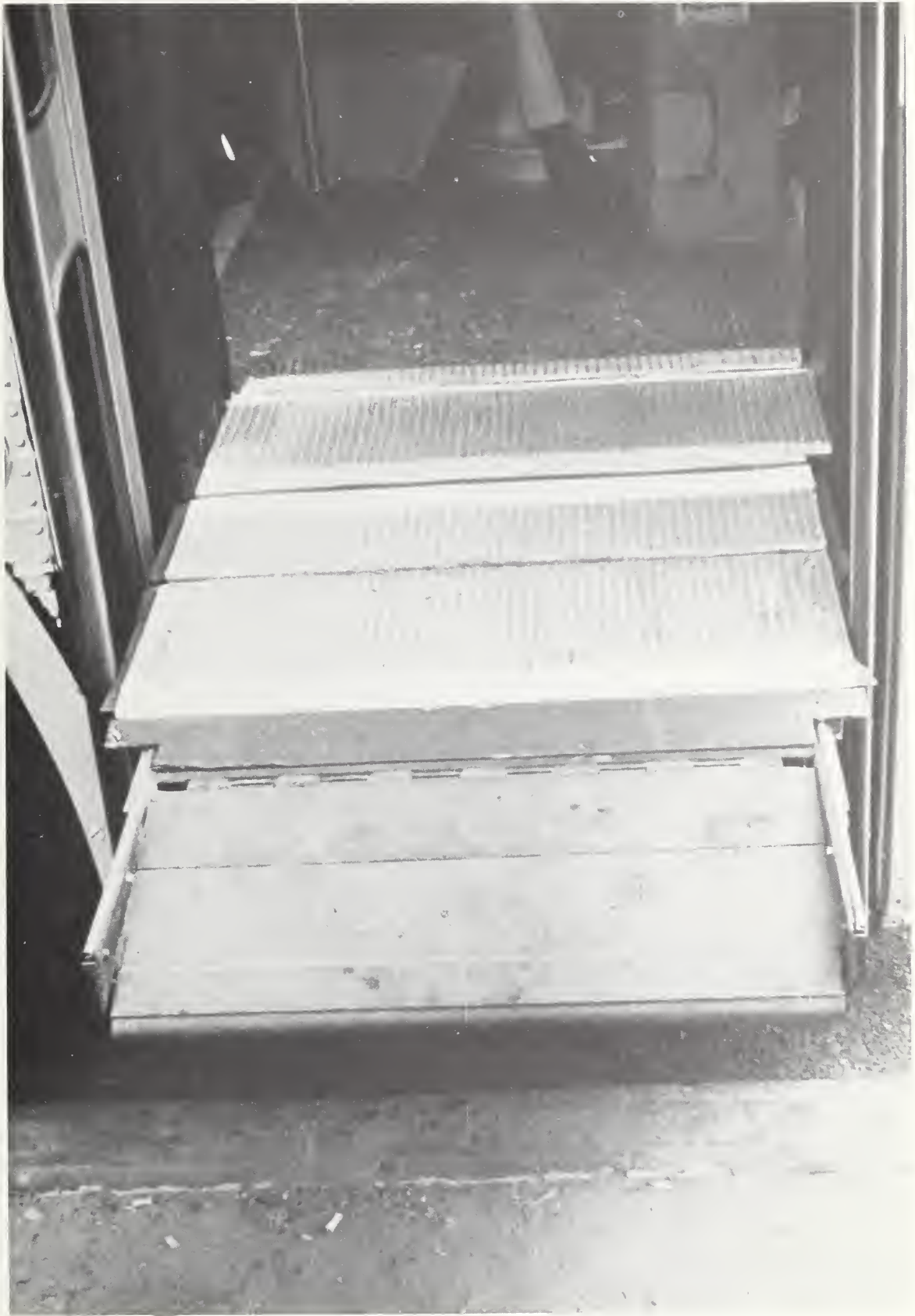
FIGURE 4-14 LIFT PLATFORM AT BUS FLOOR LEVEL
