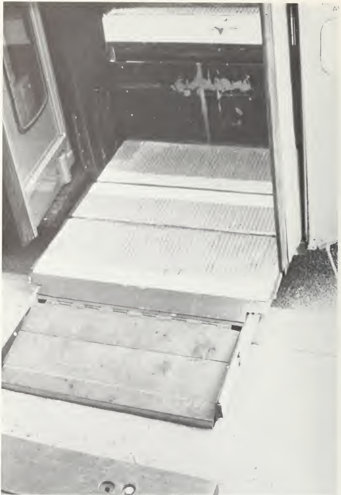
FIGURE 4-13 LIFT PLATFORM AT CURB LEVEL
