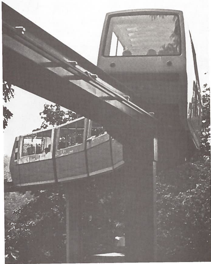
Figure A-30. Photograph of Unimobil II Vehicles and Guideway (Courtesy: Universal Mobility, Inc.)
