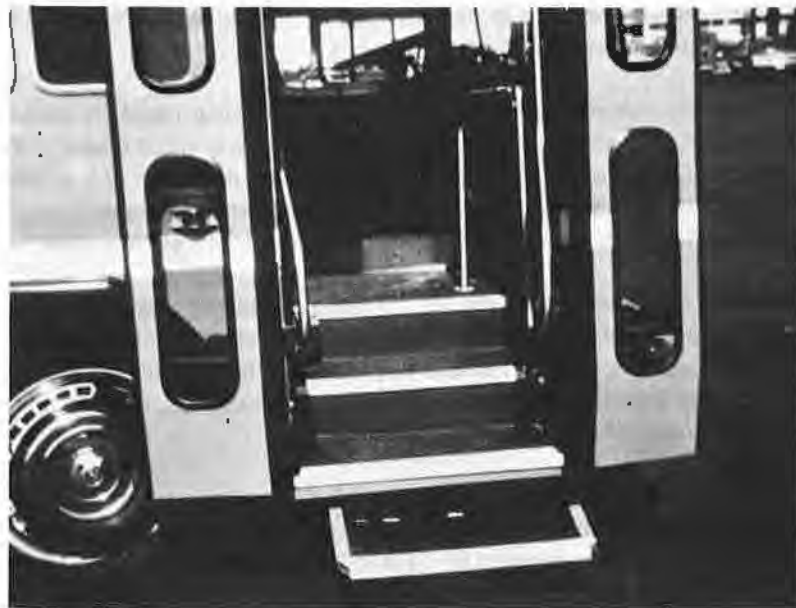
Figure 16. Low, Wide Steps Provide Ease of Boarding - Naugatuck Valley, Connecticut
