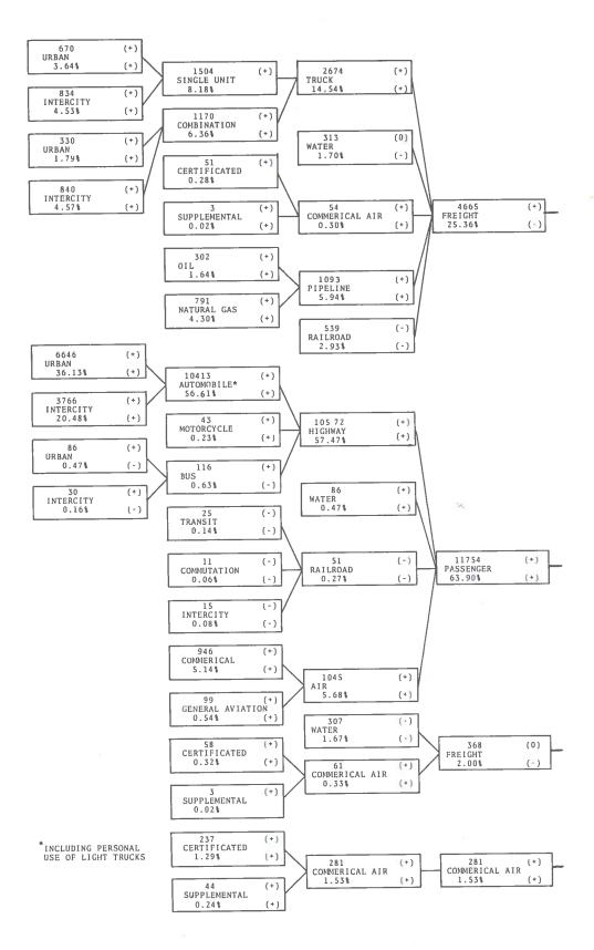
Figure S-1. Breakdown Chart of the U.S. Transportation System and Its Energy Consumption in 1972
