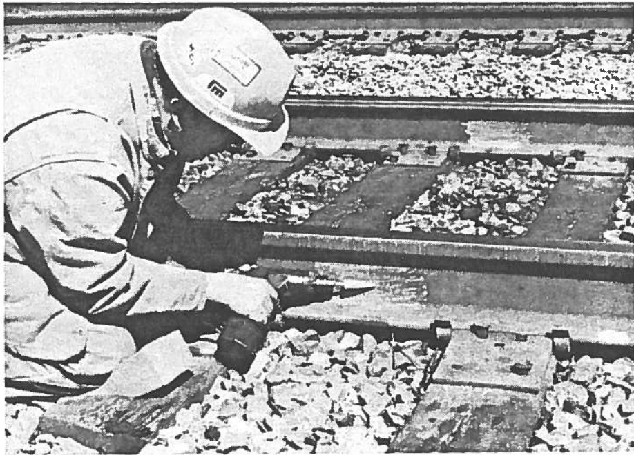
Figure D-2. Fine Grinding of Rail for Strain Gauge Application
