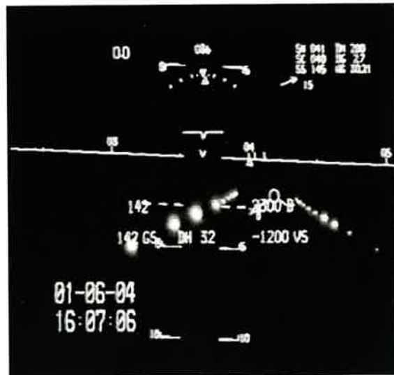
Figure 3.1-3c – UV Light Image Superimposed Over Flight Control Vector & Other Symbology
