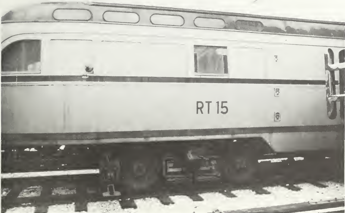
FIG. 137. THE GRINDING BLOCK ARRANGEMENT UNDER THE TRUCKS OF THE TTC (TORONTO) RAIL GRINDING CAR.
