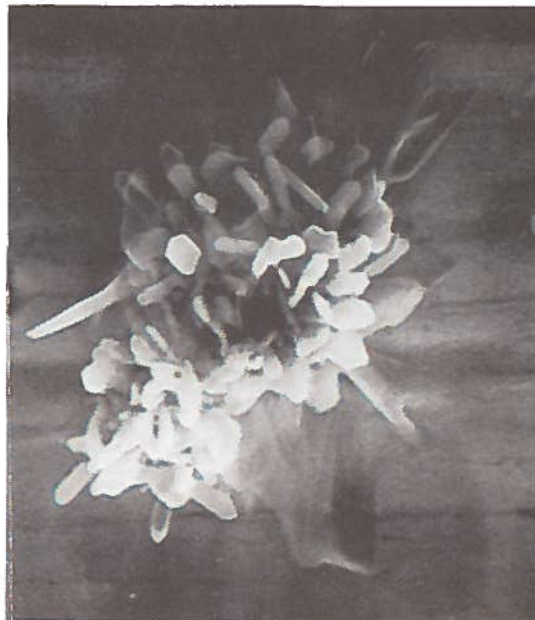
Figure 7. 10-μm crystal-shaped particle containing Al, Ca, Si, and S. Magnification is 10,000 x.
