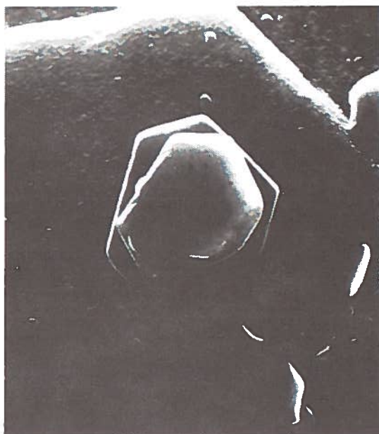
Figure 15. 9- \mu\text{m} crystalline platelets lying on a 44- \mu\text{m} platelet partially shown. Magnification is 10,000 x.
