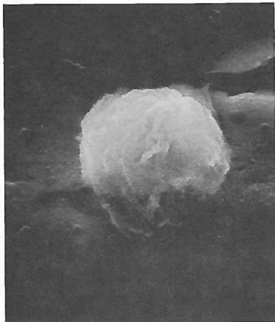
Figure 9. 5- \mu\text{m} cotton-ball-shaped particle containing Ca and S. Magnification is 10,000 x.
