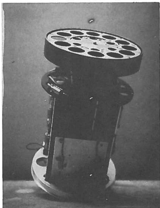
Figure 4. View of UV spectrophotometer with housing removed (showing filter wheel on top, electronics on bottom).
