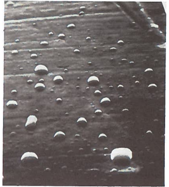
Figure 4. Large collection of ring-structure-type particles. Note lack of interaction of rings from different particles. Magnification is 10,000 x. Largest particle is about 1 \mu\text{m} in diameter.
