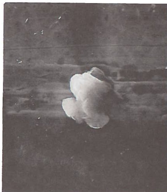
Figure 8. 3-μm amorphous particle containing Al and S.
