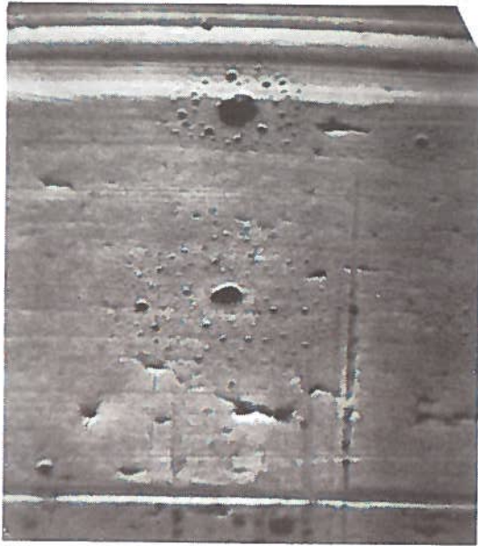
Figure 2. Ring-structure type particle. Magnification is 10,000 x. Largest particle in picture is about 0.8 \mu\text{m} .
