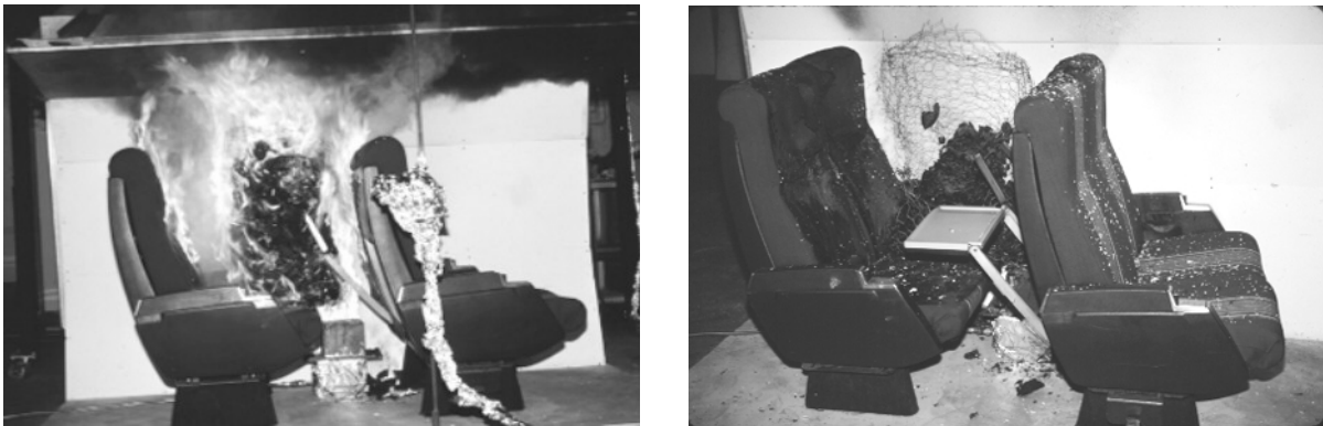
Figure A-23. Seat Assembly Test - During and After Trash Bag/Gas Sand Burner Ignition
