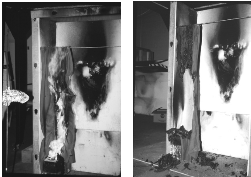
Figure A-31. Door Privacy Curtain Assembly Test (Non-Extended) - During and After Gas Sand Burner Ignition
