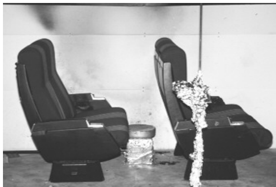
Figure A-7. Coach Seat Assembly Test - Round Gas Burner Ignition Source
