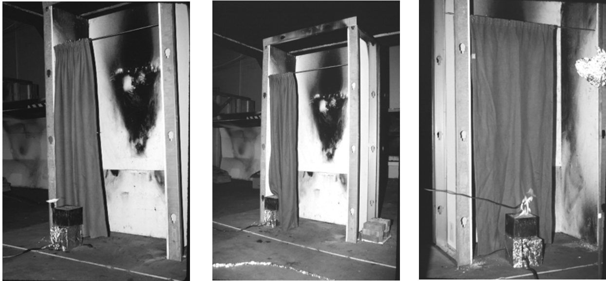
Figure A-14 b. Door Privacy Curtain Test Configuration -Gas Sand Burner Ignition Source (3 Locations)
