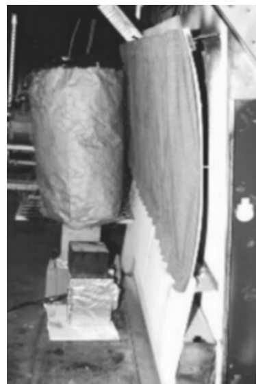
Figure A-17. Window and Drapery Tests - Trash Bag/Gas Sand Burner Ignition Source
