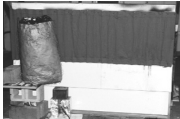
Figure A-16. Wall and Window Assembly Tests - General Configuration With Gas Sand Burner Ignition Source
