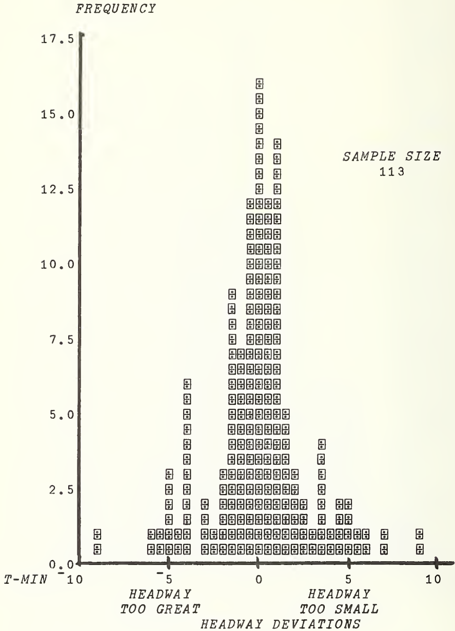
Figure 4-22 Headway Adherence Skokie Monitored Offpeak
