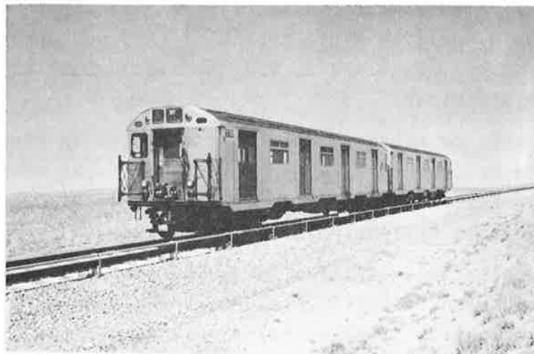
Figure 2-2 Energy Storage Cars (ESC), Modified NYCTA R-32 Cars, at TTC, Equipped with Energy Storage Flywheels
