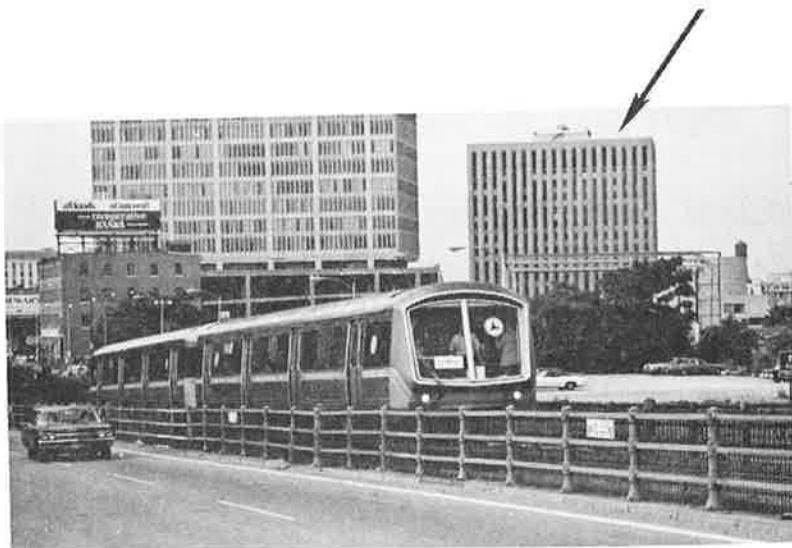
Figure 2-4 State-of-the-Art Cars (SOAC) on MBTA Red Line, TSC, Kendall Square, Cambridge, Mass., in Right Center Background
