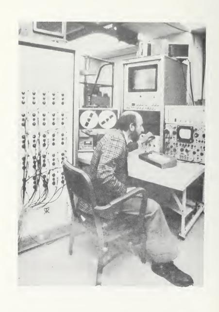
FIGURE 7. SCAN-CONTROL AND DATA-EVALUATION CONSOLE
