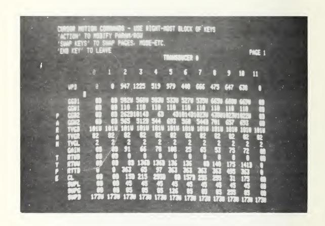
FIGURE 9. TABULAR DISPLAY OF SIGNAL-PROCESSOR PARAMETERS. Numeric Input Will Replace Or Increment Parameter Value For A Particular Transducer Number Selected By Positioning The Cursor As Shown, Or For All Transducers If Cursor Is Positioned Before Beginning Of A Row.
