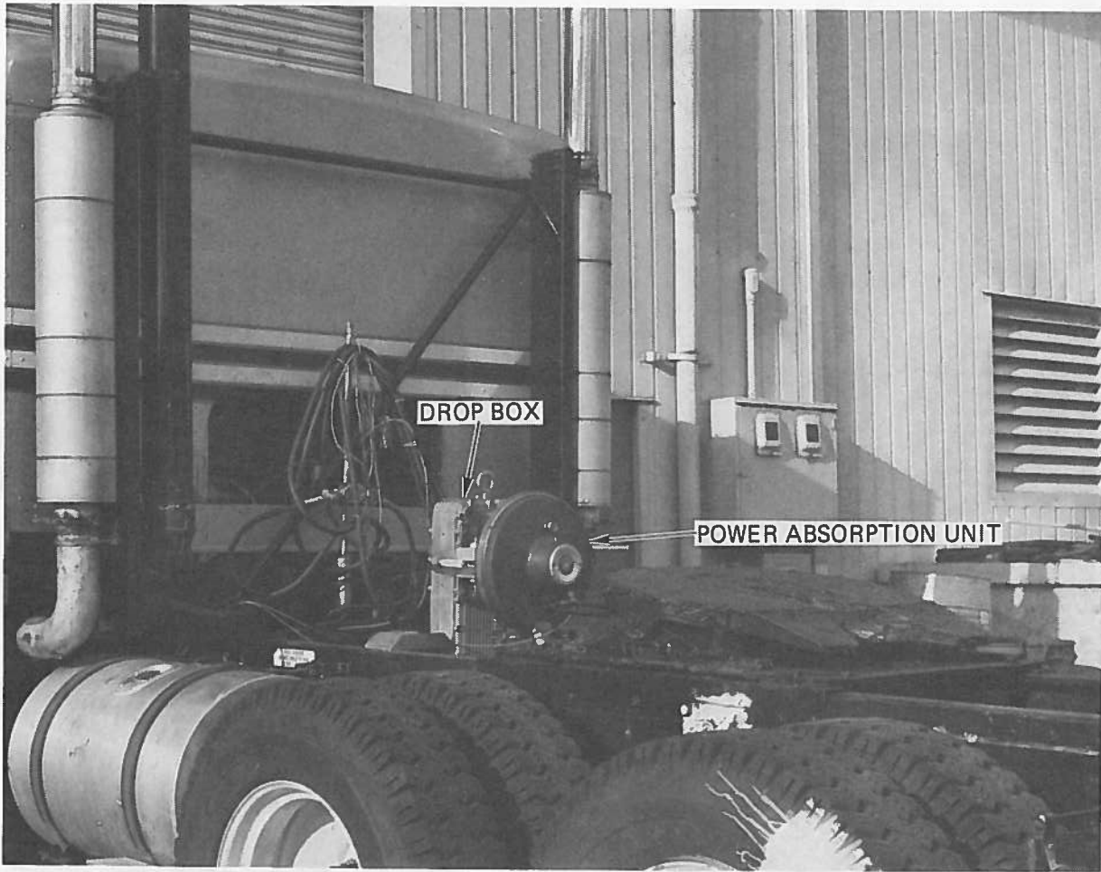
Figure 26. Dynamometer Installed on the Kenworth
