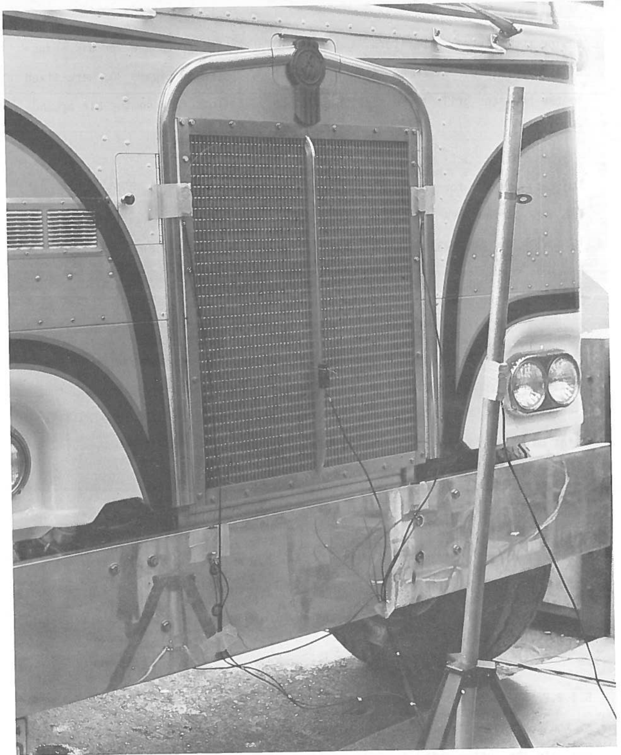
Figure 30. Cooling Test Thermocouples on the Kenworth
