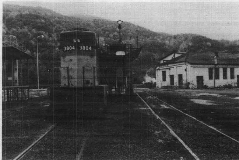
(a) Looking South at the Test Locomotive; the Test Load Cell is on the Right, the Microphones are out of the Picture to the Left; a Second Load Cell not used in the Testing Can Be Seen to the Left.
