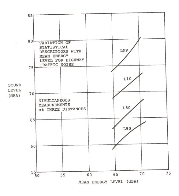
Figure 2. Variation of Statistical Descriptors With Mean Energy Level for Highway Traffic Noise.
