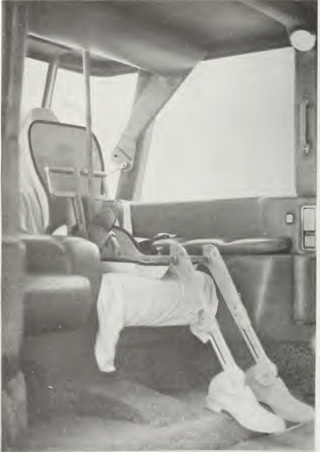
Figure 23. H-point Machine Installed in Passenger Seat of Dutcher Prototype.
