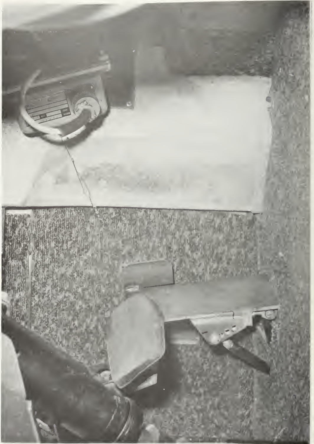
Figure 12. Throttle Position Instrumentation as Installed in Dutcher Prototype.
