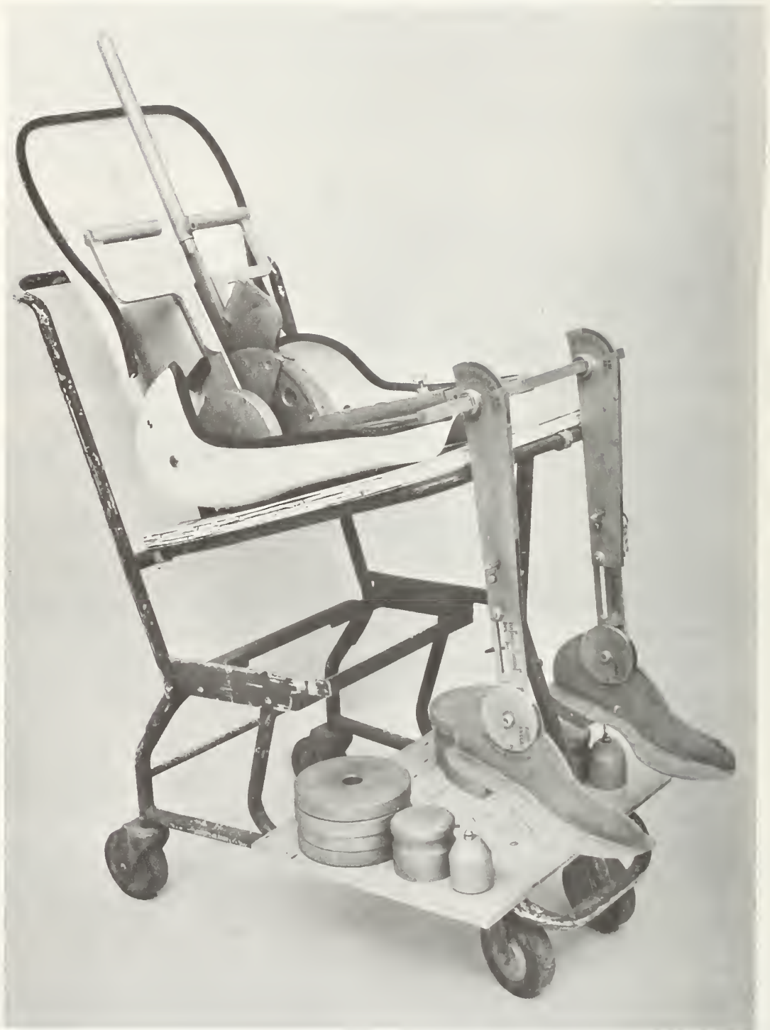
Figure 7. Three-Dimensional H-Point Machine (SAE J826b).
