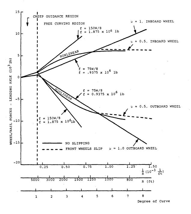
FIGURE 9. WHEEL/RAIL FORCE ON LEADING AXLE VERSUS RADIUS. COMPARISON OF LINEAR AND NONLINEAR CREEP CALCULATION. (GRAVITATIONAL FORCE NEGLECTED)
