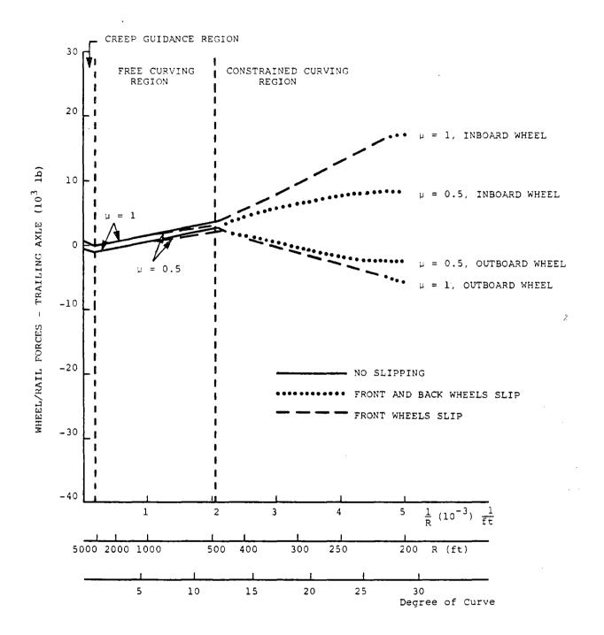
FIGURE 6. LATERAL WHEEL/RAIL FORCES ON TRAILING AXLE VERSUS RADIUS OF TRACK
