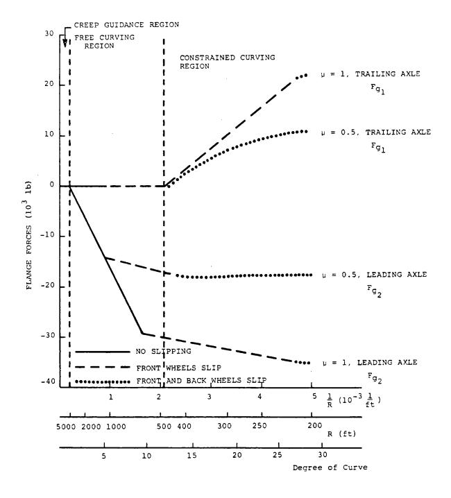
FIGURE 4. FLANGE FORCE ON INNER AND OUTER AXLE VERSUS RADIUS OF TRACK
