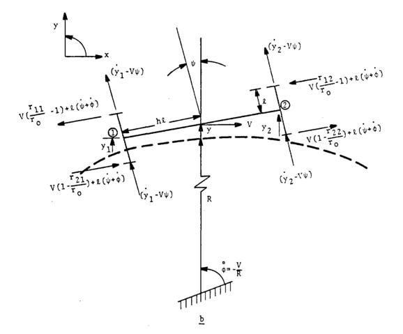
FIGURE 1. STEADY STATE CURVING MODEL OF RIGID TWO-AXLE TRUCK SHOWING CREEP VELOCITY COMPONENTS
