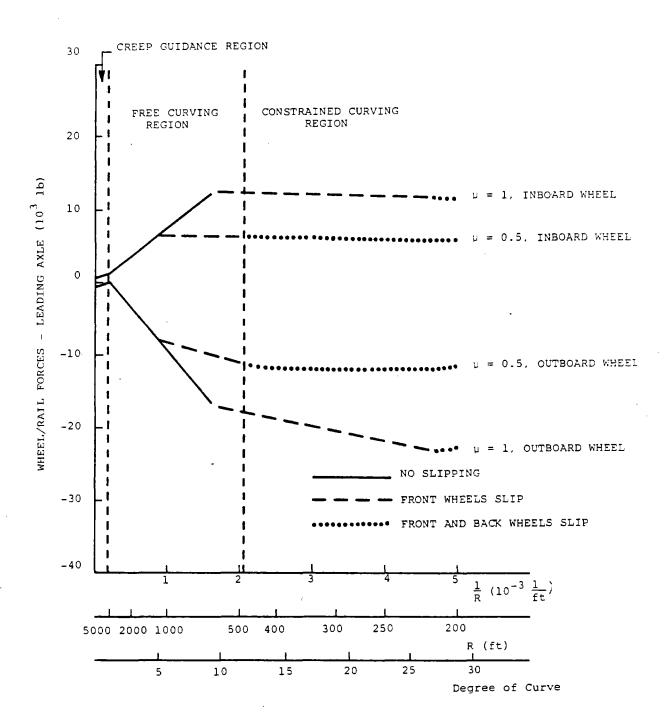
FIGURE 5. LATERAL WHEEL/RAIL FORCES ON LEADING AXLE VERSUS RADIUS OF TRACK
