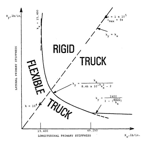
FIGURE 12. RANGE OF VALIDITY OF FLEXIBLE AND RIGID TRUCK MODELS IN TERMS OF PRIMARY STIFFNESS (h = 1.41,  $\ell$  = 28.2",  $\alpha$  = 0.05)
