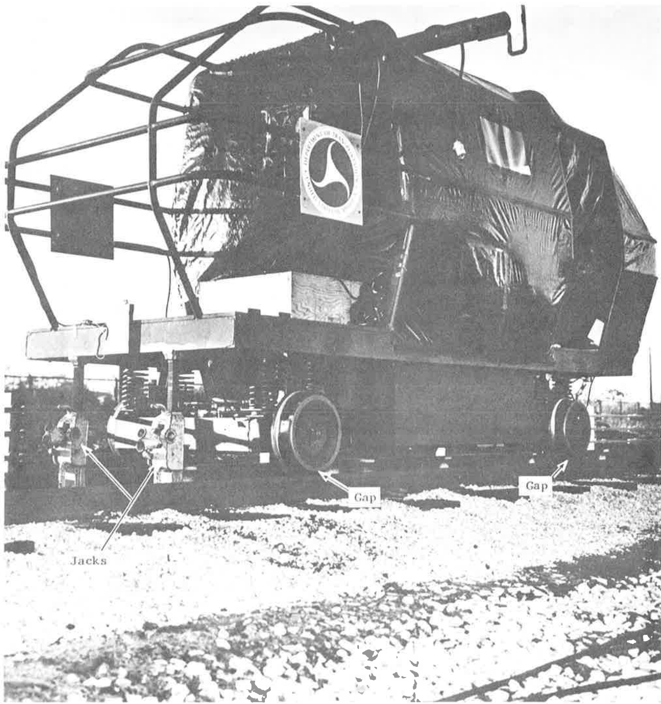
Vehicle in Jacked Position
