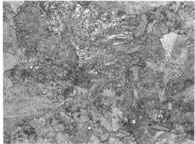
B. 112-LB RAIL MICROSTRUCTURE (500X)
