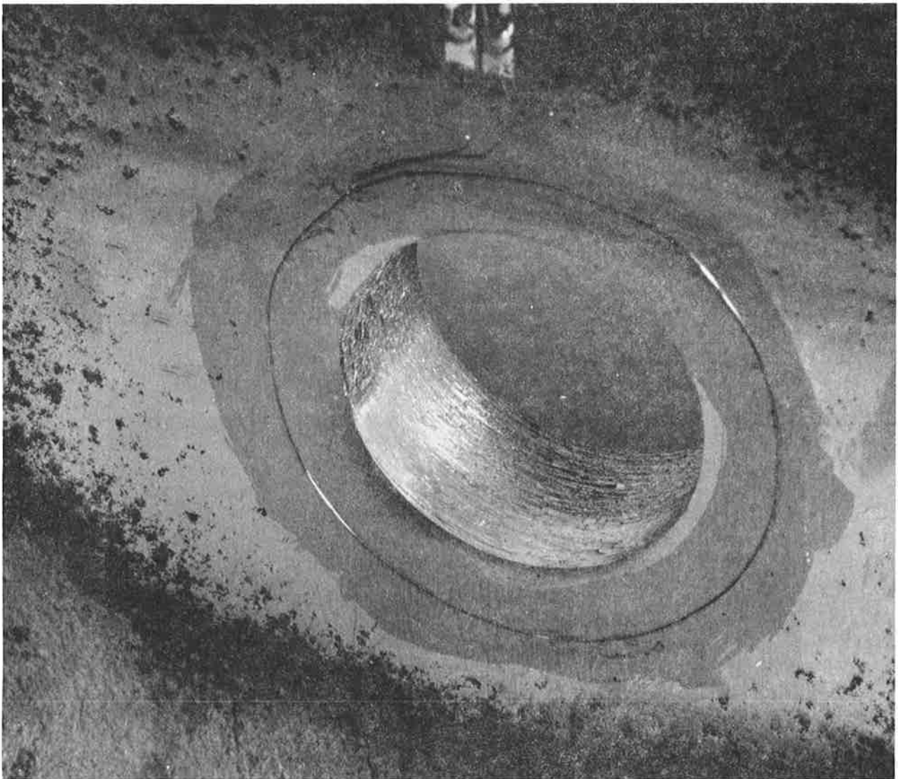
Figure 24.—Crack Wire Circuit
