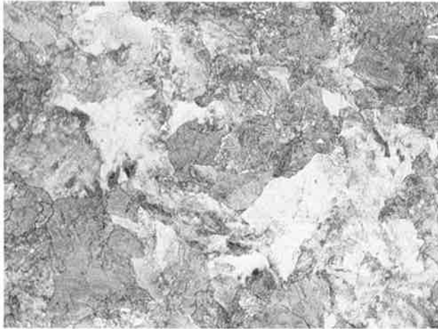
A. 1075 PLATE PEARLITIC MICROSTRUCTURE (500X)
